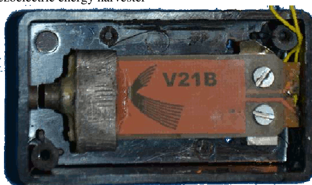
Figure 11. Bi-stable nonlinear piezoelectric energy harvester
