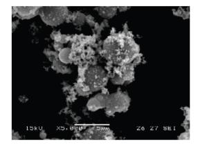
Figure 2: Left, particle size distribution of dirhenium-heptasulfide from our production. Right, scanning electron microscope image of dirhenium-heptasulfide particles (round).
