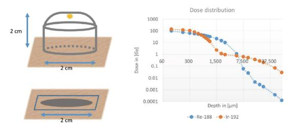
**Figure 1:** Right, dose at different skin depth for Rhenium-188 versus Iridium-192 for a comparable total dose of 65 Gy within the first 1.5mm. Simulations were performed using NRC's VARSKIN 5.2 software [14]. Left, schematics of simulated scenarios with VARSKIN.
