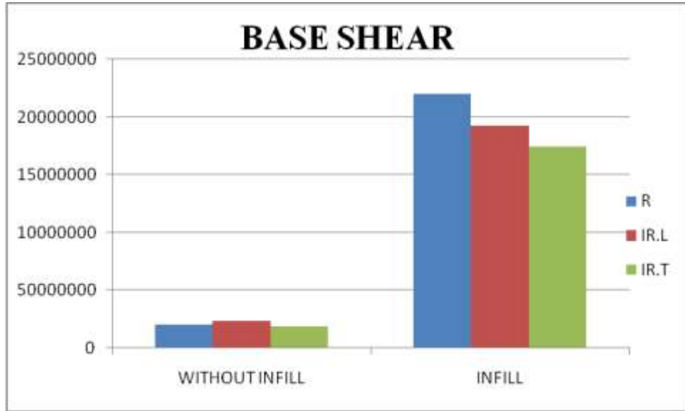
Fig 14 Base shear of all models with and without infill
