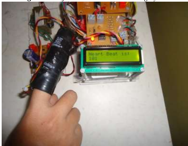
Fig.8: Hardware and Measurement of Heartbeat.
