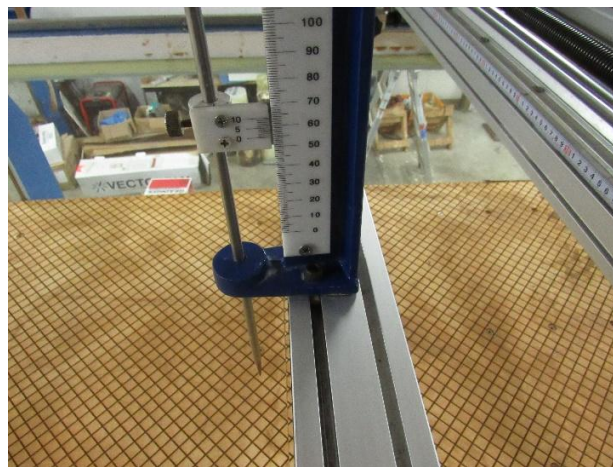
Figure 3.4 The point gauge for water depth measurements
