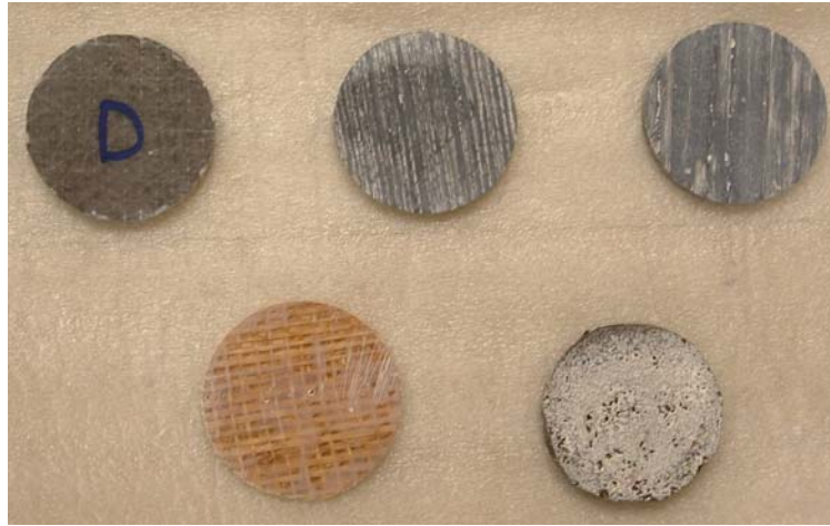
Figure 4.5 Samples of bridge deck, natural fiber, deck with epoxy wearing surface
