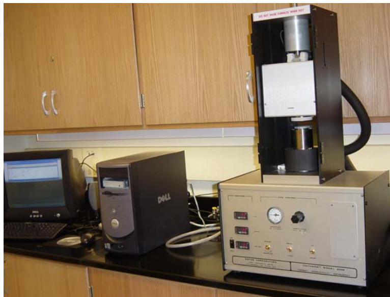
Figure 3.1 Experimental set up of Unitherm 2022
