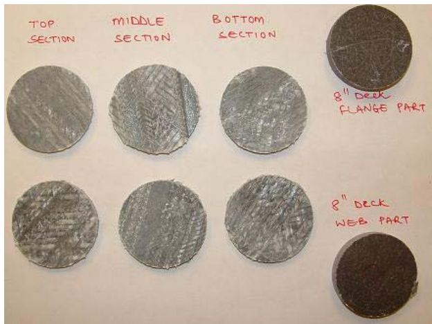
Figure 4.9 Samples prepared from web and flange sections of Prodeck 8
