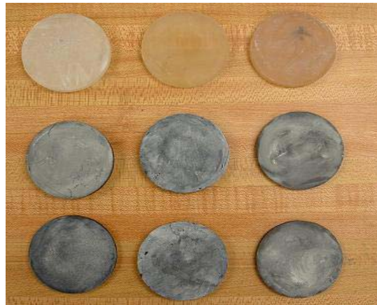
Figure 4.1 Samples of Epoxy, Vinyl ester and Polyester resins on top row; samples with different particulate sizes of graphite powder additive, chopped carbon fiber additives in bottom two rows
