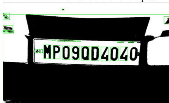
Figure 6; Building Boxes over Characters and numbers by bounding box method
