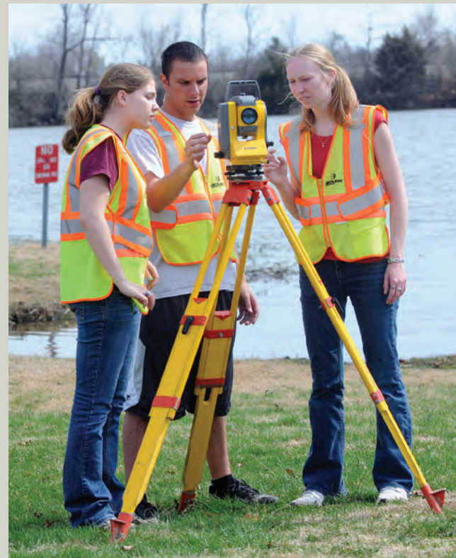
Surveying has been an essential civil engineering course since the university's founding. Students learn how to determine boundaries of land and water using measuring devices and mapping systems to make planning decisions.
