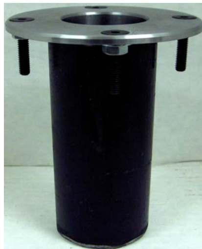
Figure 3.13. The 6-inch Bolt Cup Installed in the Wall and Roof of the Blue Room.
