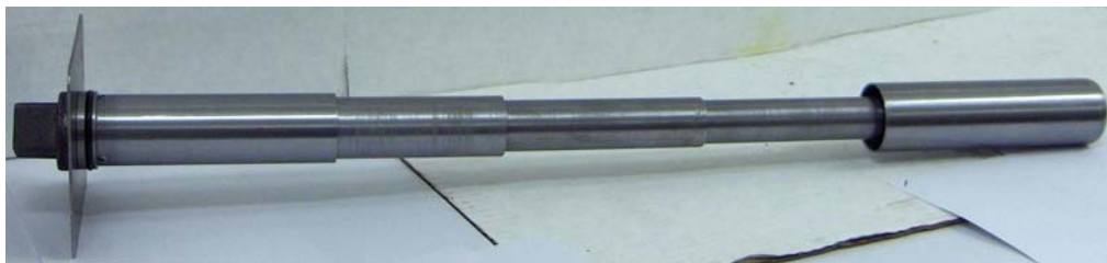
Figure 3.14. The 2 ft Rockbolt with a 4.5 x 4.5-inch Plate and 6-inch Cup in its Fully Expanded State.
