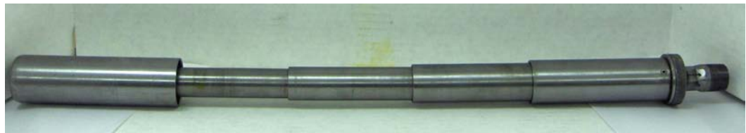
Figure 3.11. The 2 ft Collapsible Drill Steel in its Fully Extended State.
