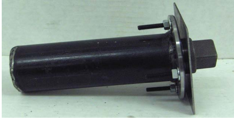
Figure 3.15. Rockbolt Model in its Fully Collapsed State within the Steel Cup.
