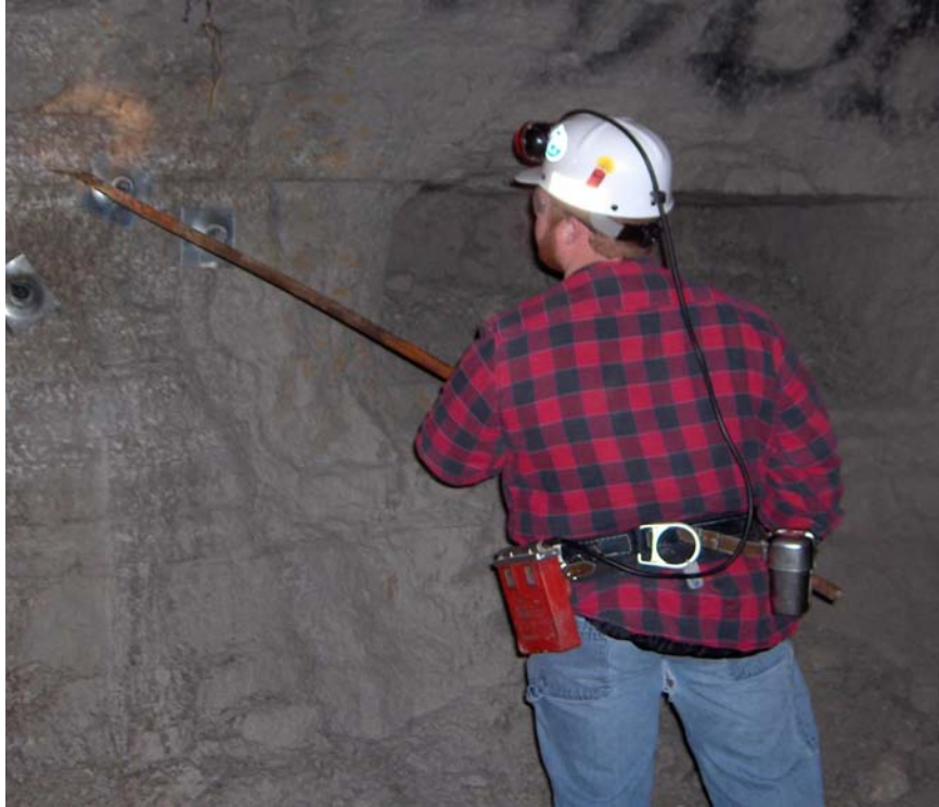
Figure 4.18. A Participant is Scaling Loose Rock During the Rockbolting Contest at the Missouri S&T Experimental Mine.
