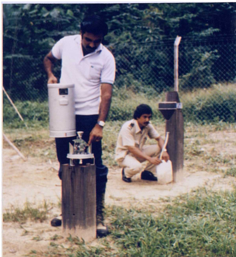
Plate 4.2 Recording and storage raingauges installed in BEW
