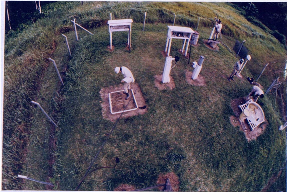
Plate 4.1 Climate station in Berembun Experimental Watershed
