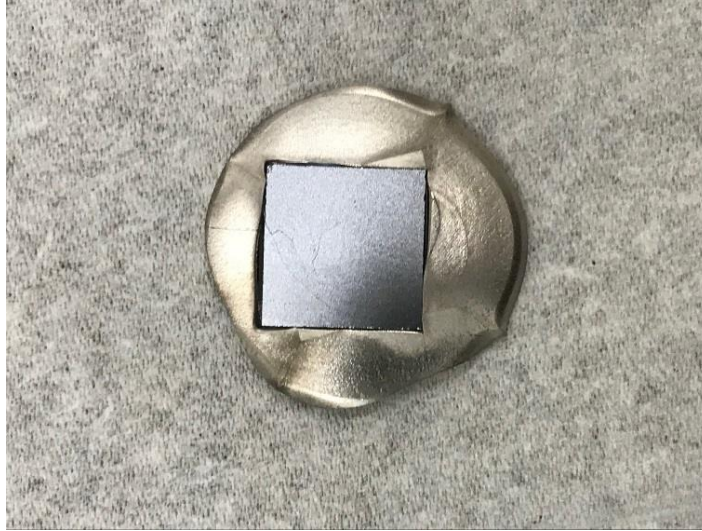
Figure 4-32: Zr-BMG TPF at 340 C with 3 minutes hold and 150 Kg load.
