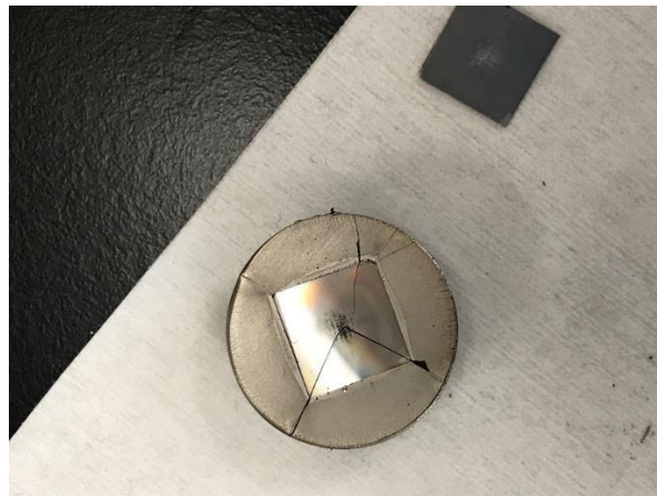
Figure 4-30: Zr-BMG TPF at 340C with 250 Kg.
