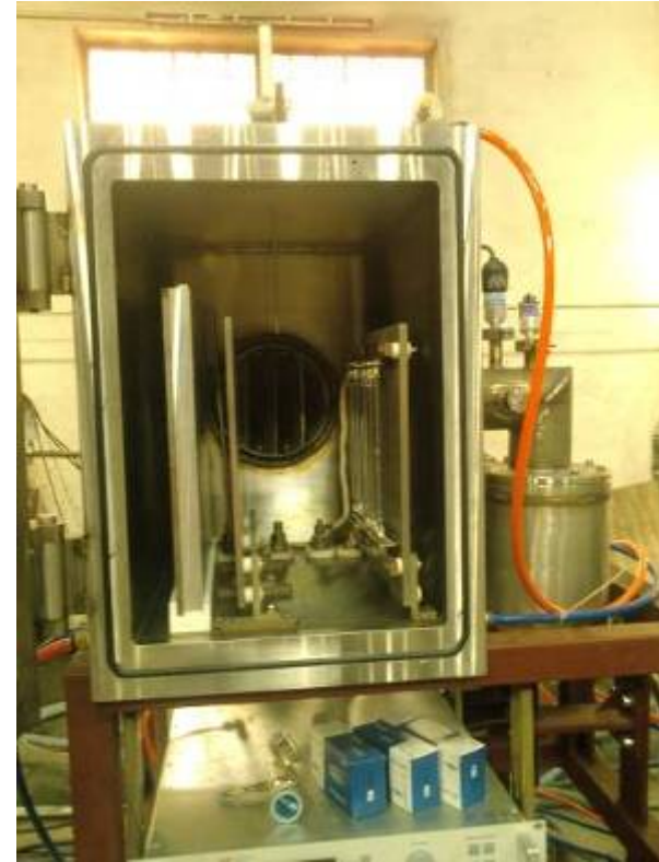
The magnetron sputter equipped in my lab which can prepare large area thin films sized 1200 \times 1000 \text{ mm}^2 . Using this sputter we complete the research for low-cost preparation of amorphous Si thin film solar cells.
