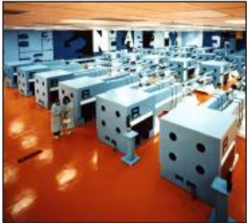
OMEGA – 24 beams, 4 kJ, 15 TW (LLE 1980)
