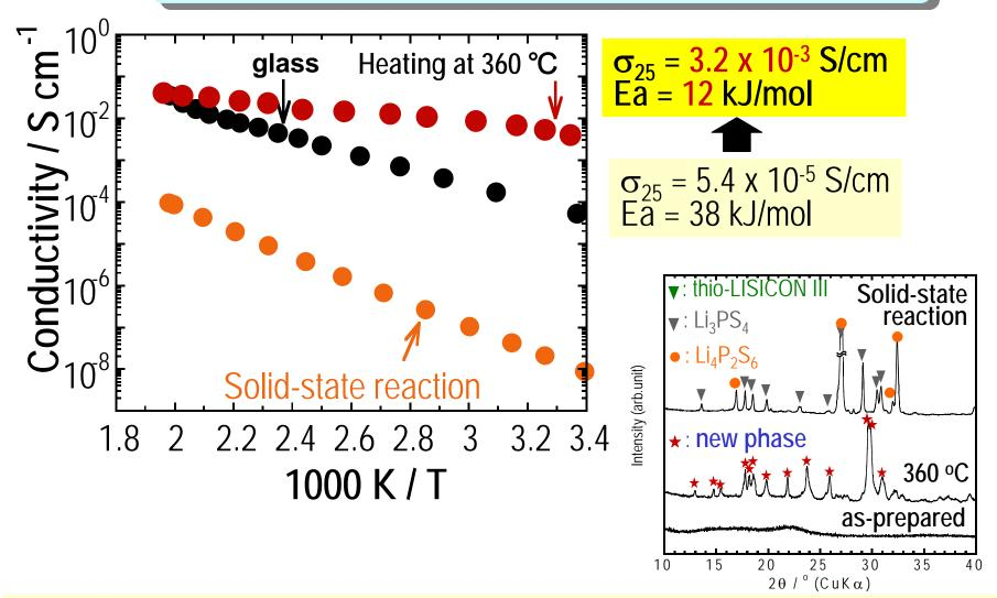
The formation of superionic metastable phase is the most remarkable advantage of glass-based solid electrolytes. All-solid-state lithium secondary batteries using  $Li_2S-P_2S_5$  glass-ceramics
