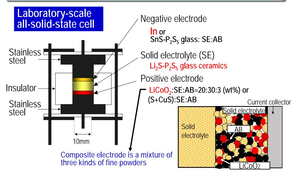
Ionic and electronic conduction paths through SE and conducting additives to active materials
