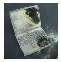
There are serious safety problems present in lithium ion secondary batteries using flammable organic liquid electrolytes.
