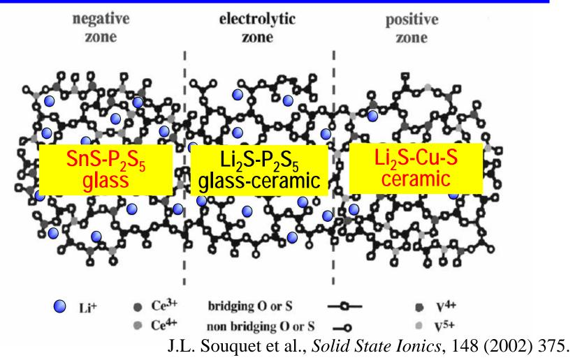
The glassy monolithic cell is expected to facilitate smooth solid-solid contact between electrolyte and electrode, and very promising as a future all-solid-state battery.
