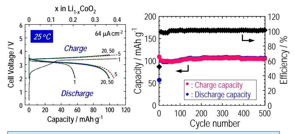
Excellent cycle performance with no loss of capacity up to the cycle number of 500
