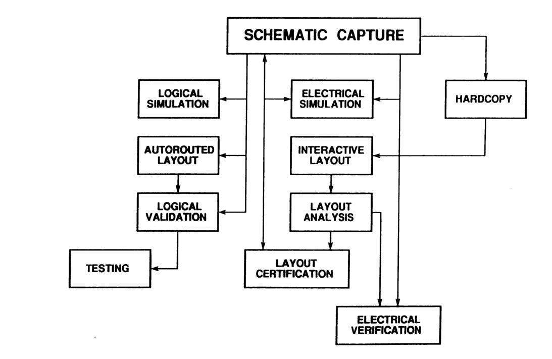
Figure 1. Process Flow for Analog IC Design
