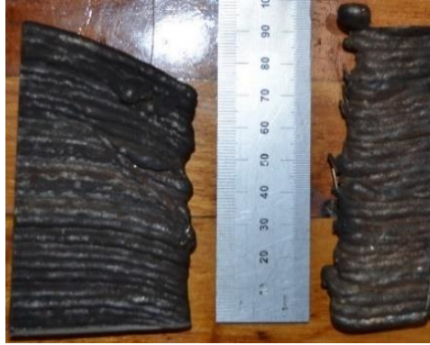
Figure 2.3 : Two ends of the real sample (start welding, right) (end welding, left)
