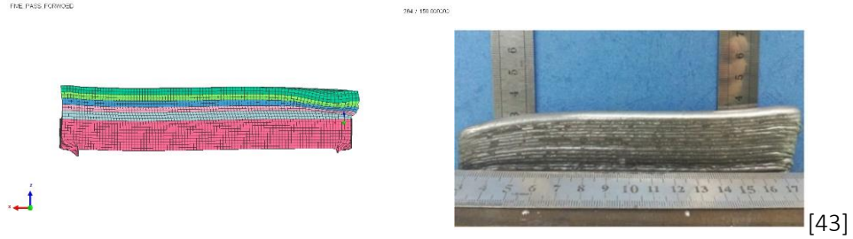
Figure 2.26 : Distortion after printing (real, bottom; simulated, top) for forward path
