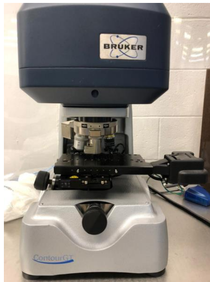
Figure 1: Scanning whit light interferometer
