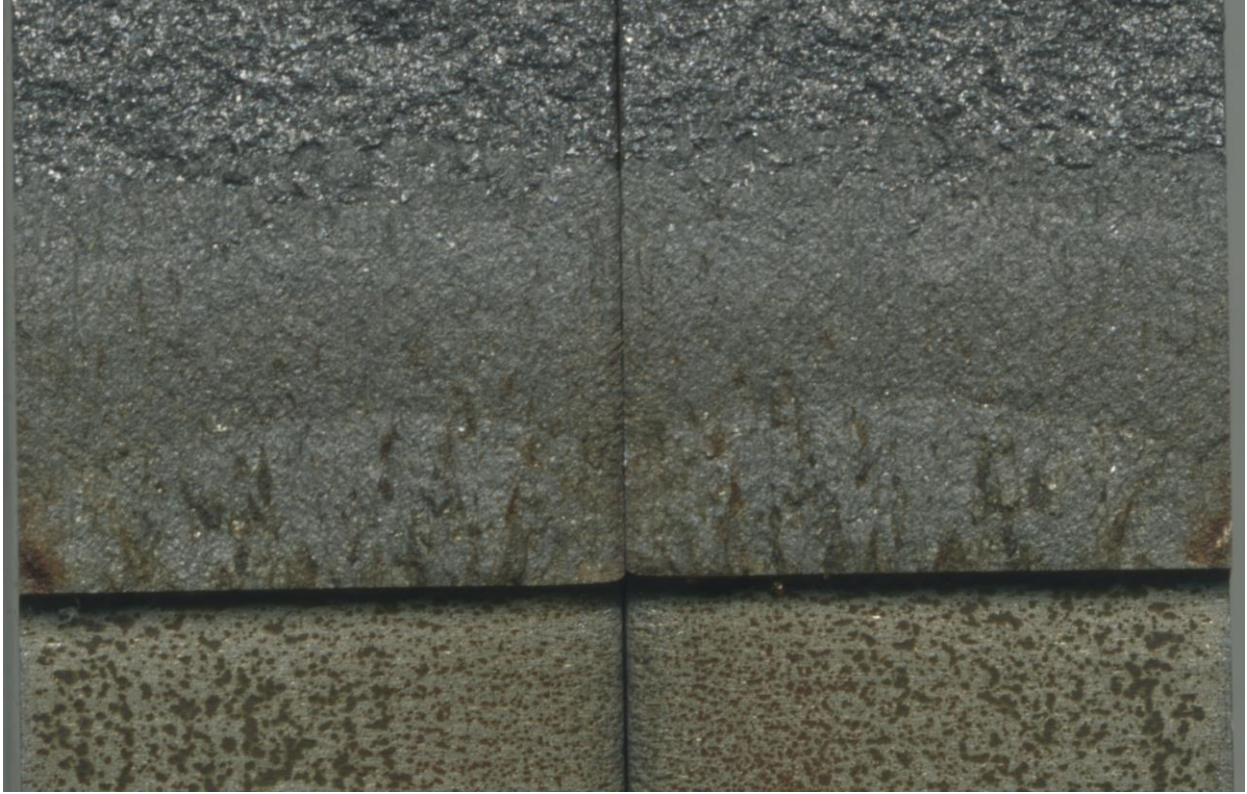
Figure 76 – Fatigue/fracture surface for HH 3A tested at R=0.33 .
