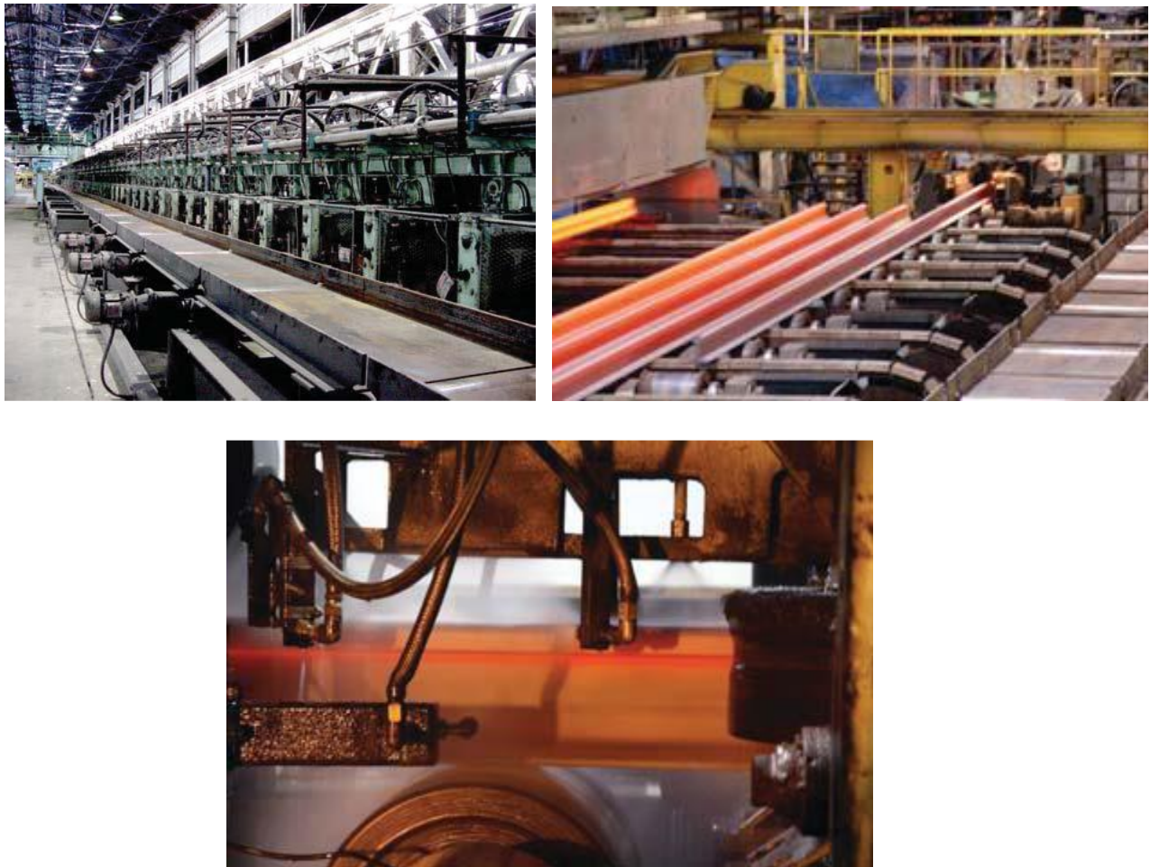
Figure 3 – Head hardening facility at ArcelorMittal, Steelton.
