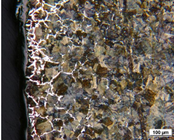
Figure 18 – LOM photomicrographs of Sample 4 from CF&I77 rail as viewed at the outer edge of the sample.
