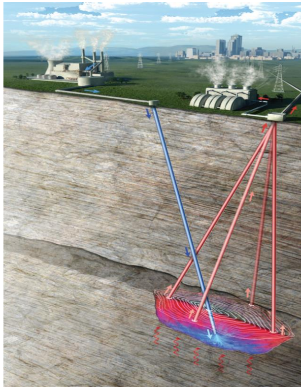
Figure 1–1 Illustration of s\text{CO}_2 injection into a geothermal reservoir for heat mining and above-the-ground geothermal energy utilization.
