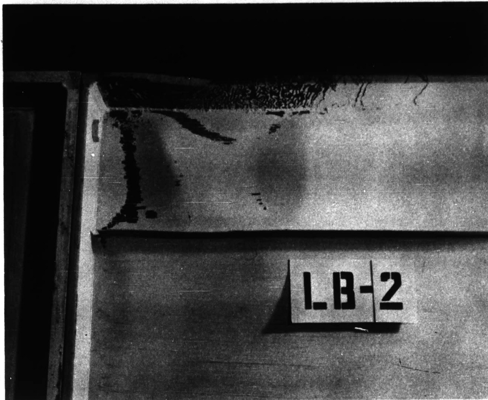
Fig. 30 Yielding in Side Panel, Near Side (Specimen LB2)
