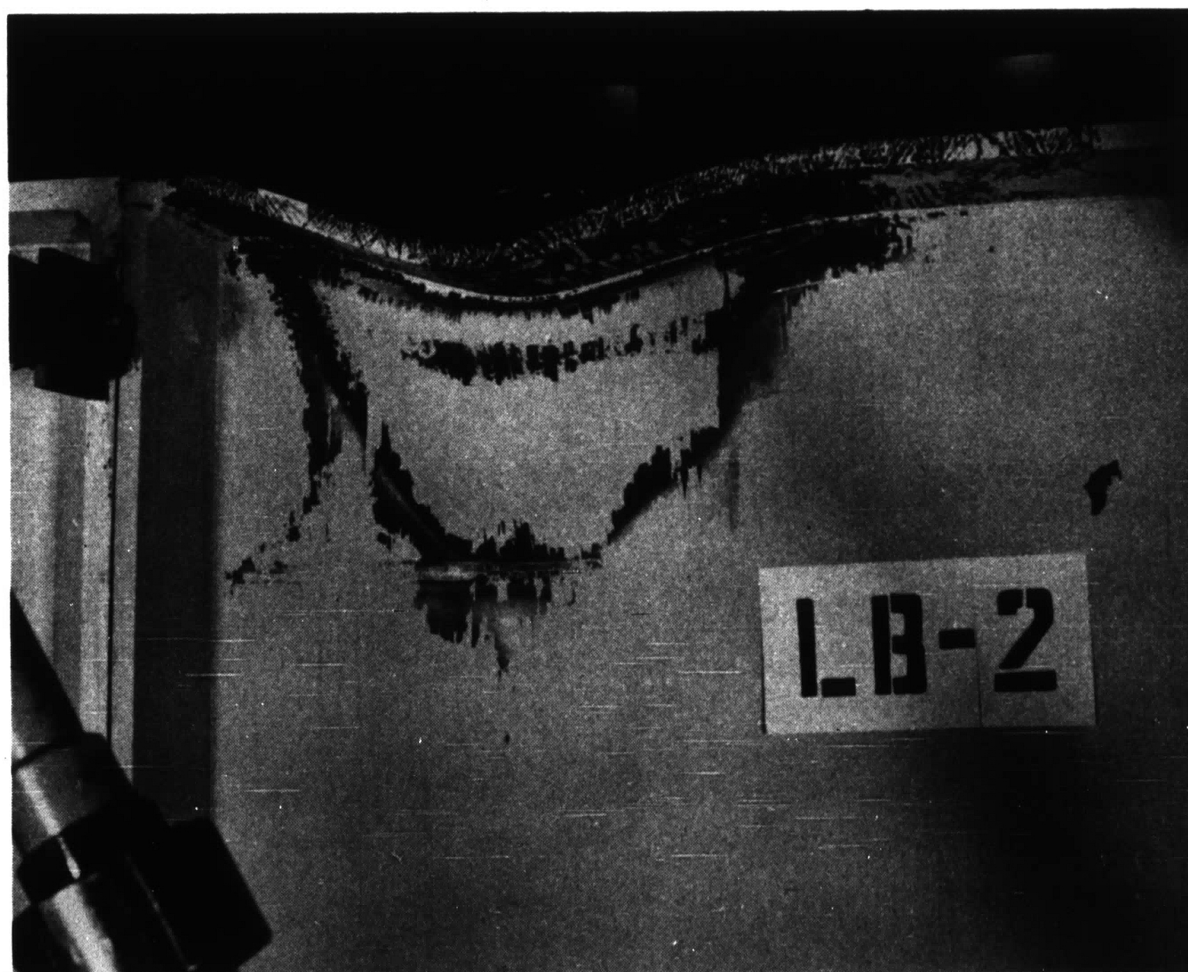
Fig. 31 Vertical Buckle, Far Side (Specimen LB2)
