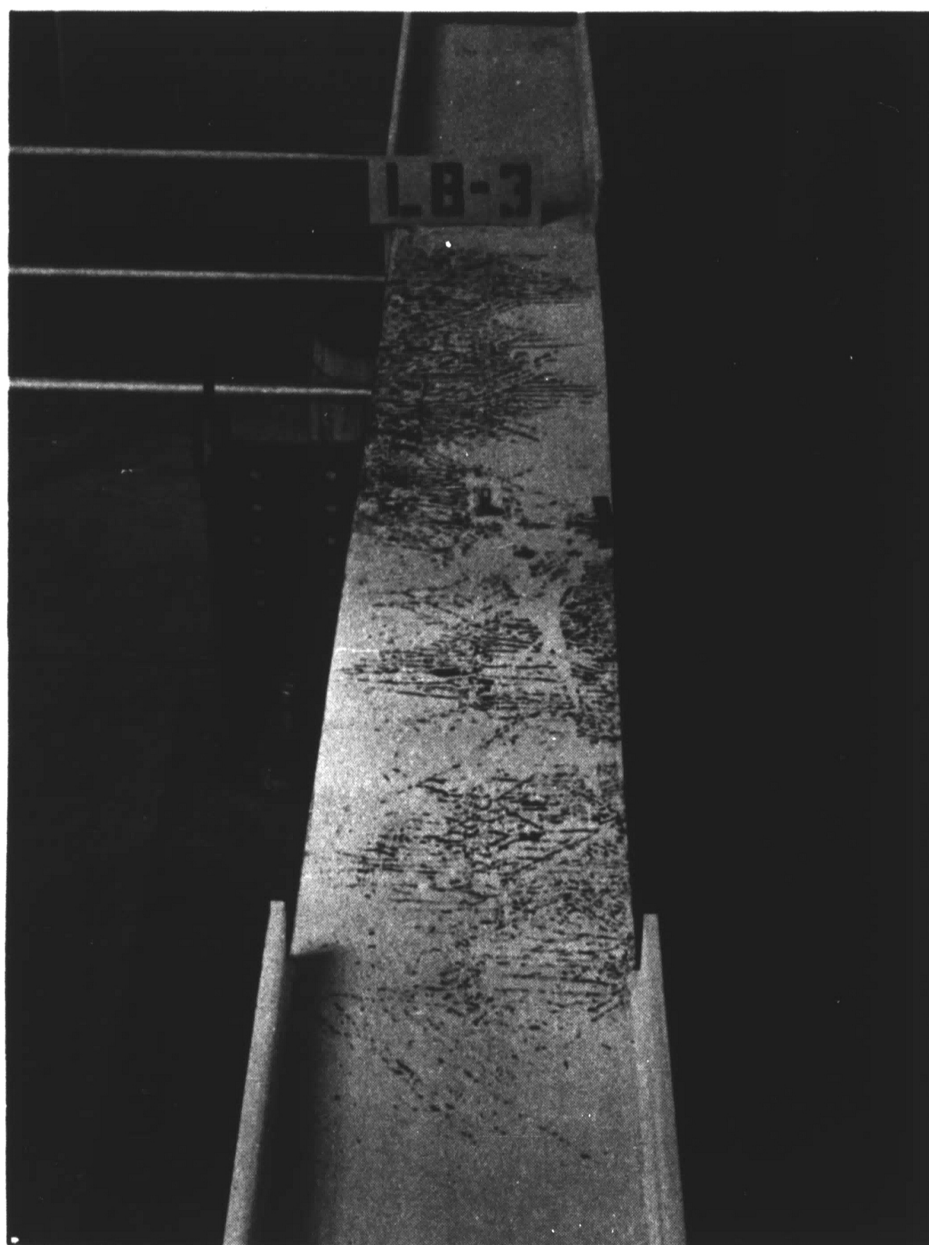
Fig. 34 Yield Pattern on Top Surface of Compression Flange (Specimen LB3)
