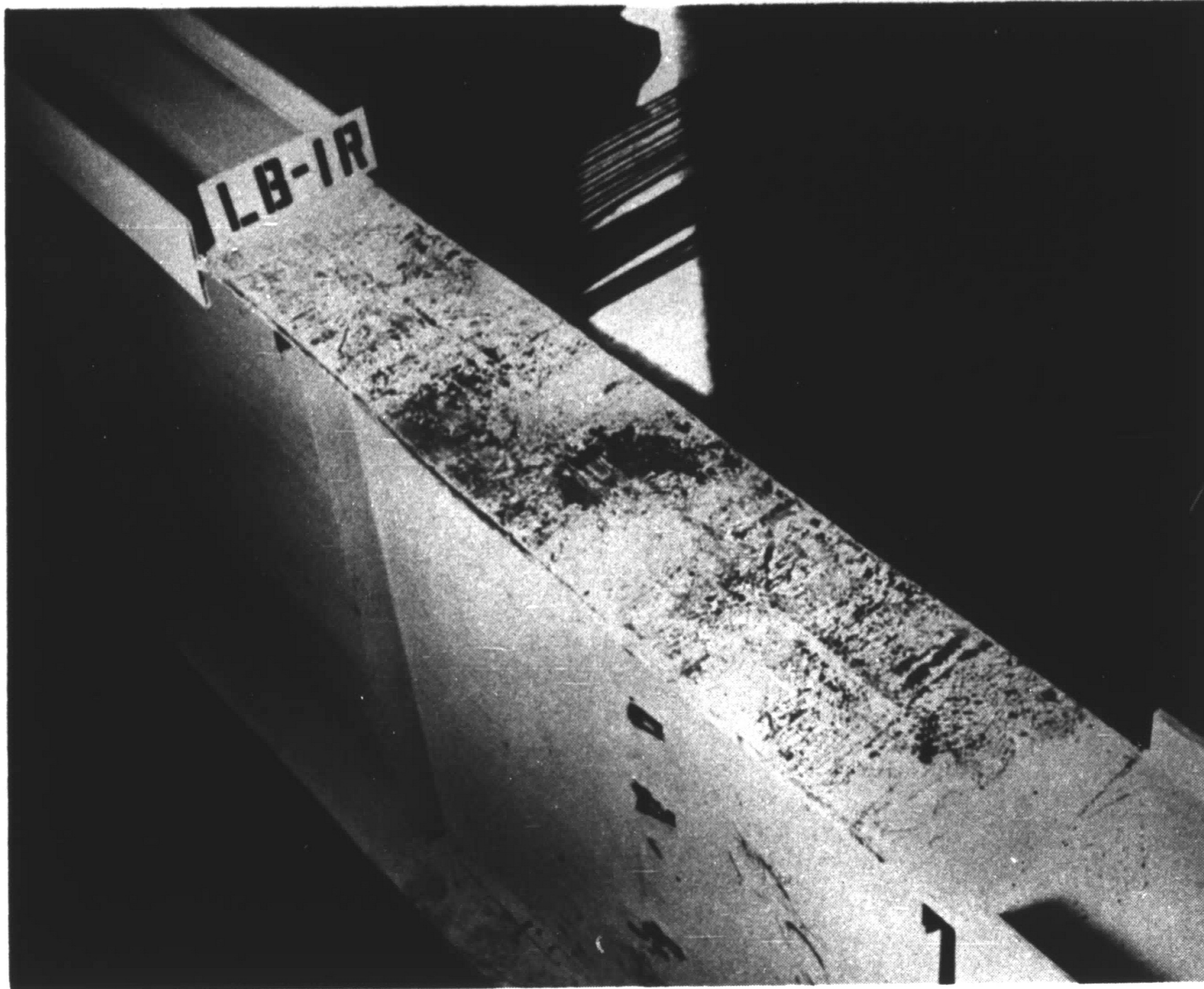
Fig. 28 Yield Pattern on Top Surface of Compression Flange (Specimen LB1)
