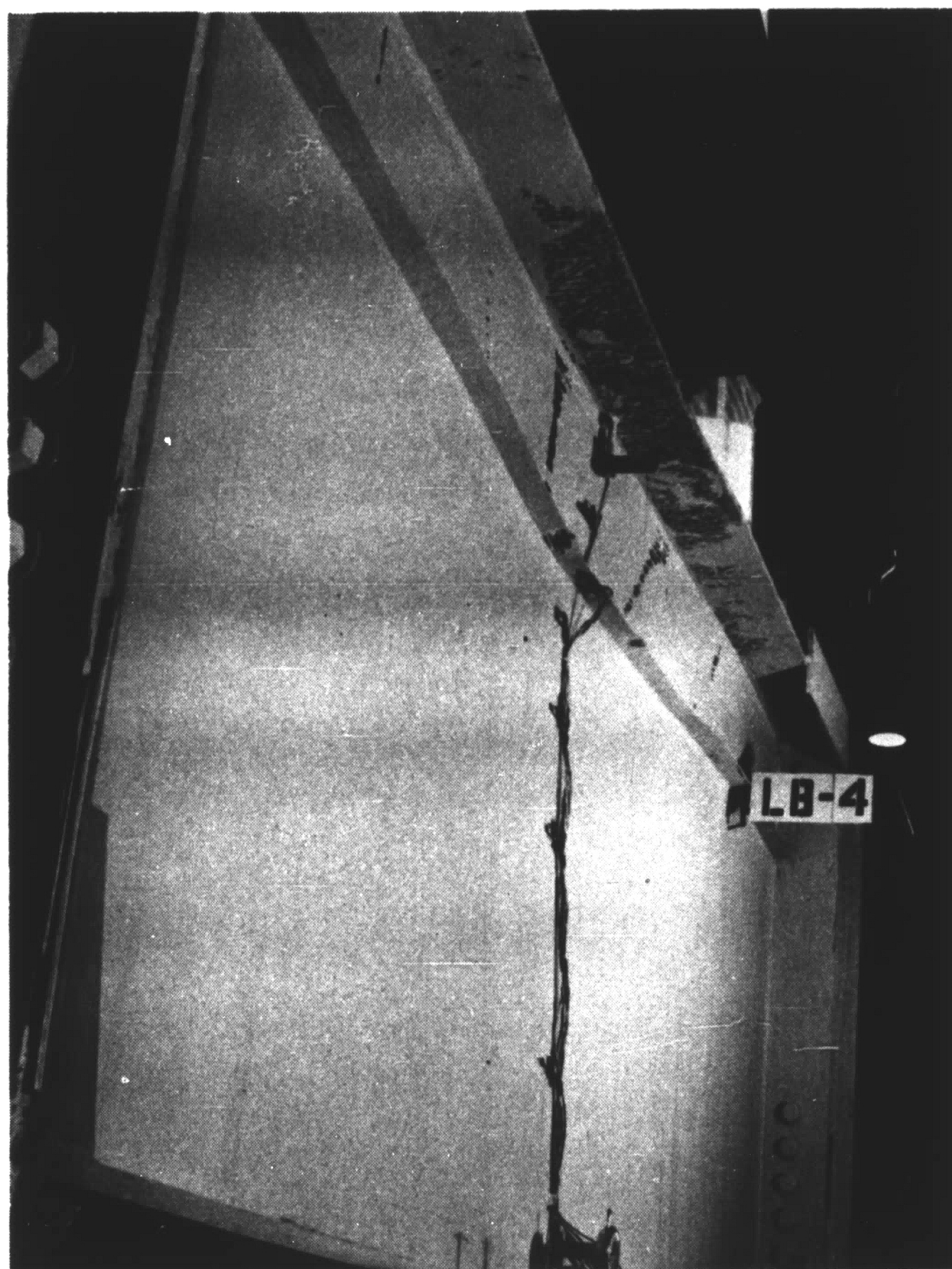
Fig. 35 Test Panel After Ultimate Load, Near Side (Specimen LB4)
