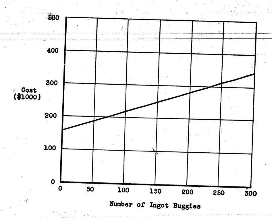
COST OF HAVING INGOT BUGGIES AVAILABLE (At output of 3,000,000 ingot tons per year)
