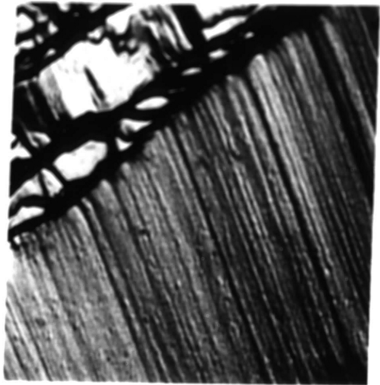
Figure 20: Electron fractographs revealing parallel fracture markings. (a) Evidence of fine parallel lines superimposed on the \gamma matrix faceted fracture surface. 10,000X. (b) Increased magnification of a region containing parallel fracture marking in order to resolve individual lines. (Spacing approximately 600Å) 23,000X.
