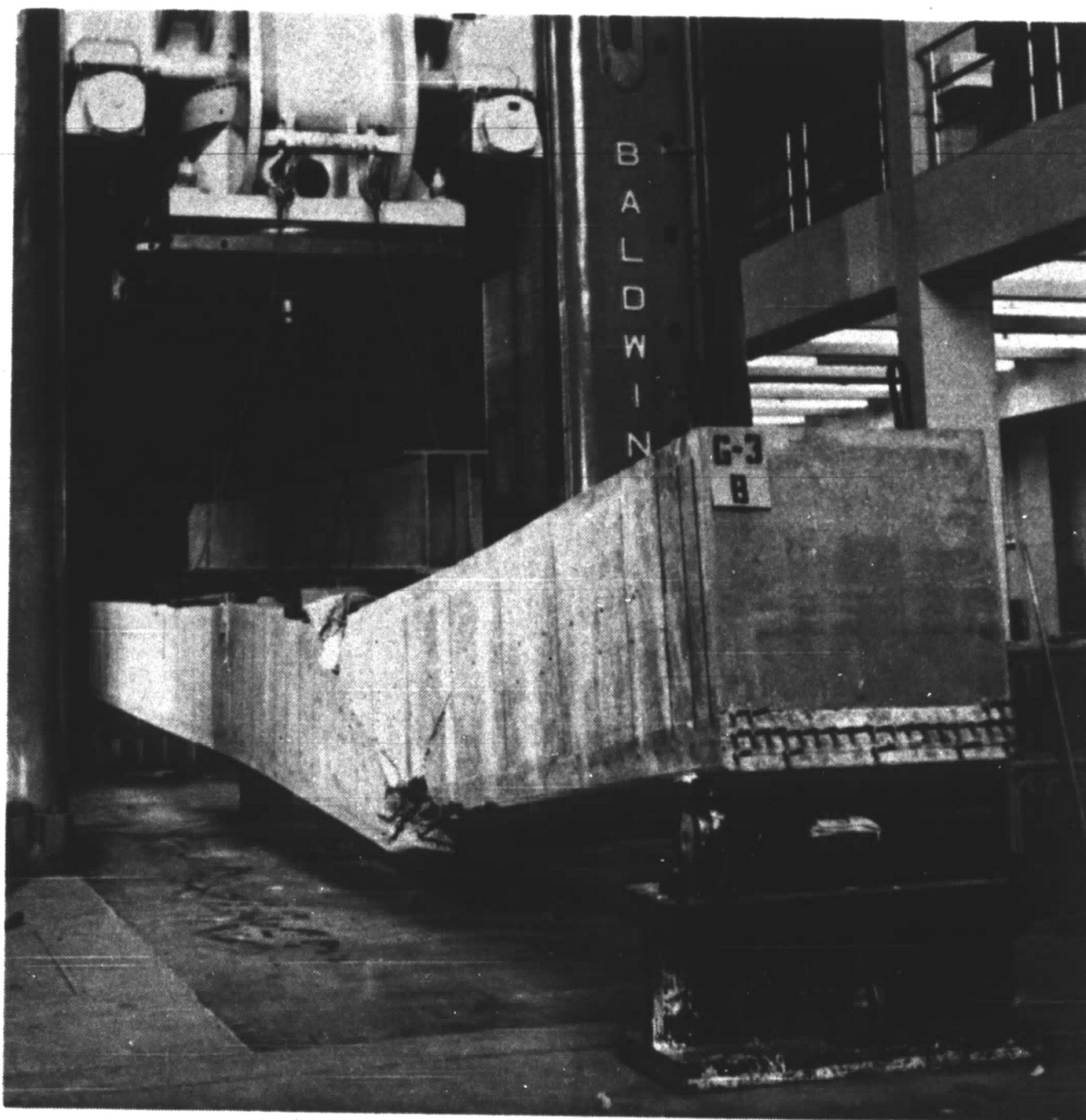
b. B Shear Span After Failure
