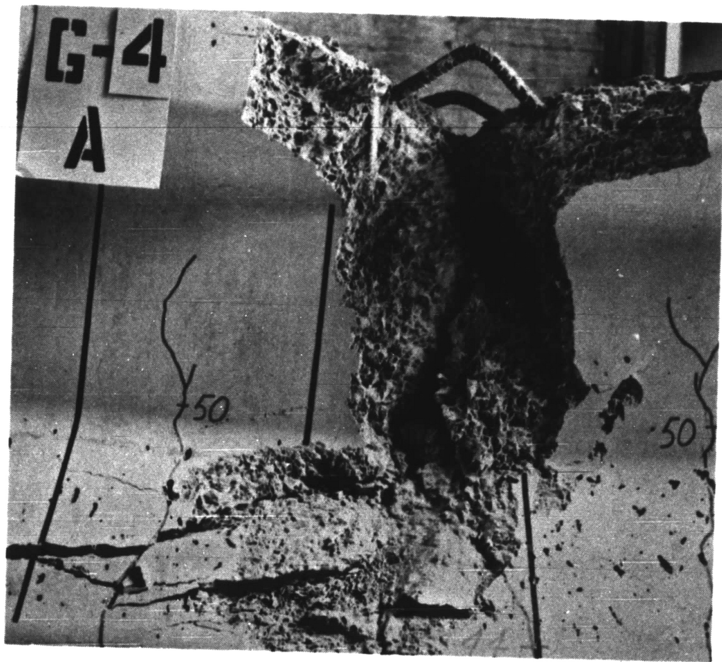
b. View of Center Region of Beam After Flexural Failure
