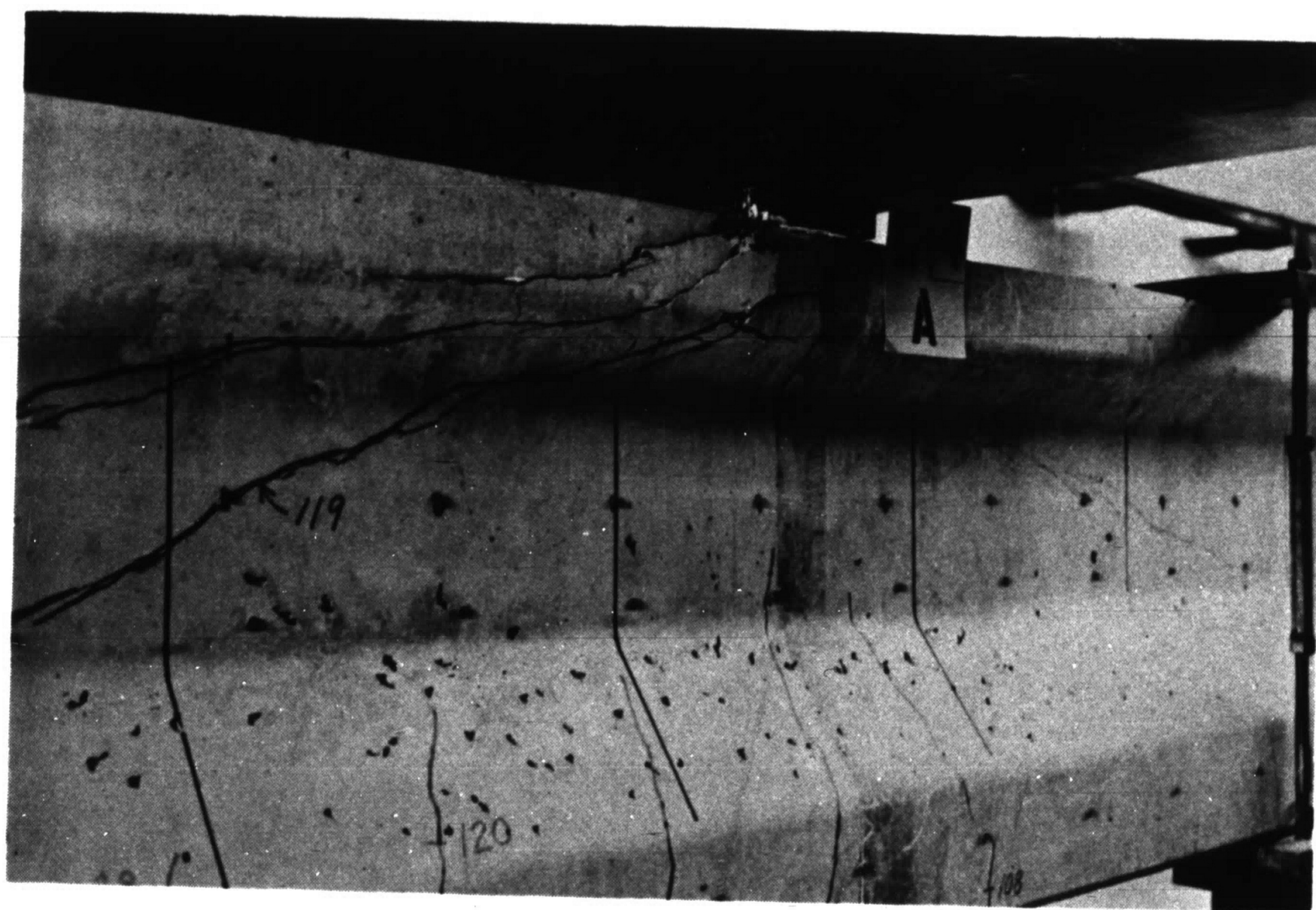
b. A Shear Span After Failure
