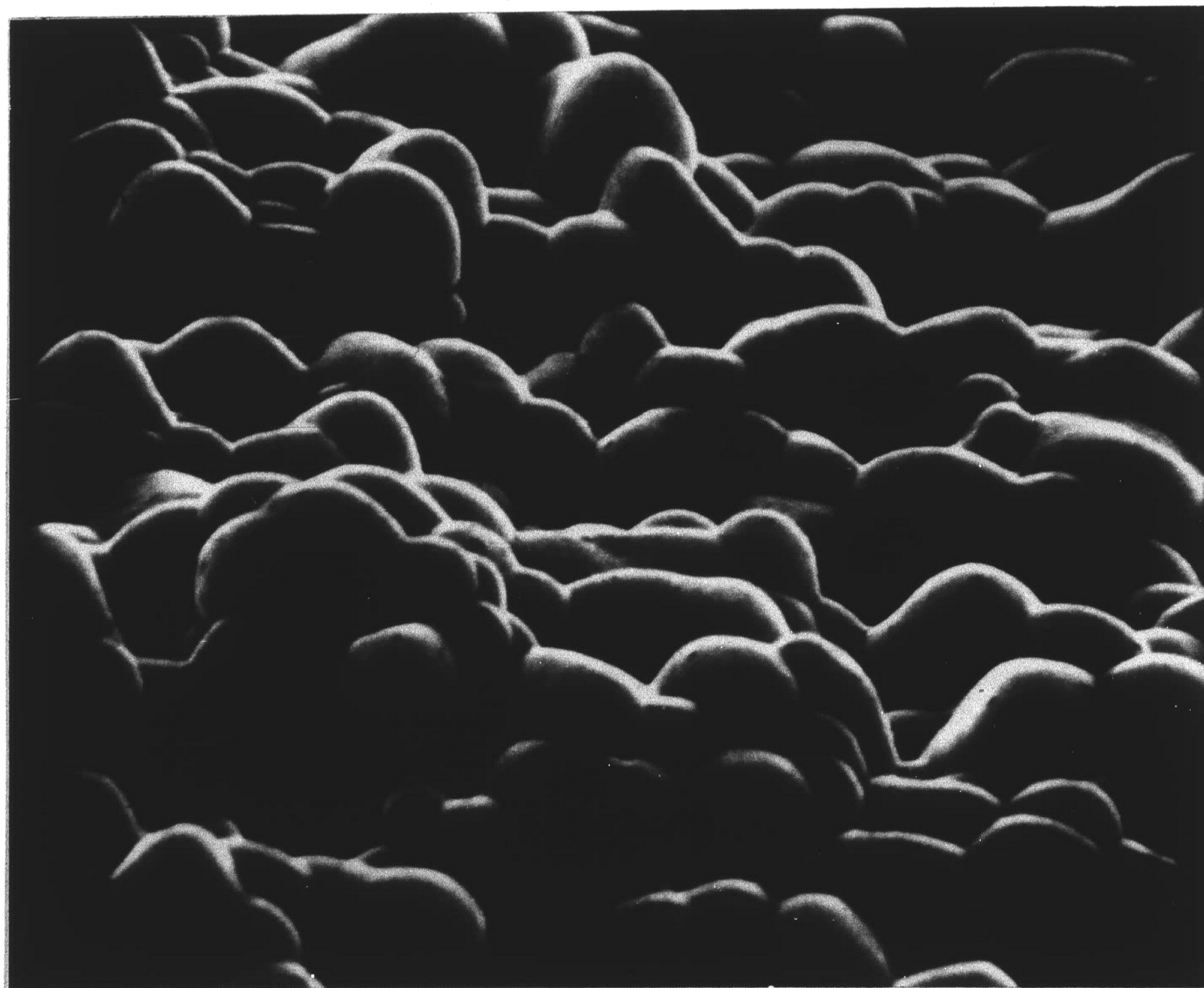
FIGURE 4 SCANNING ELECTRON MICROGRAPH OF A FRACTURED PLZT SURFACE WHICH HAS BEEN THERMALLY ETCHED (10,000X)
