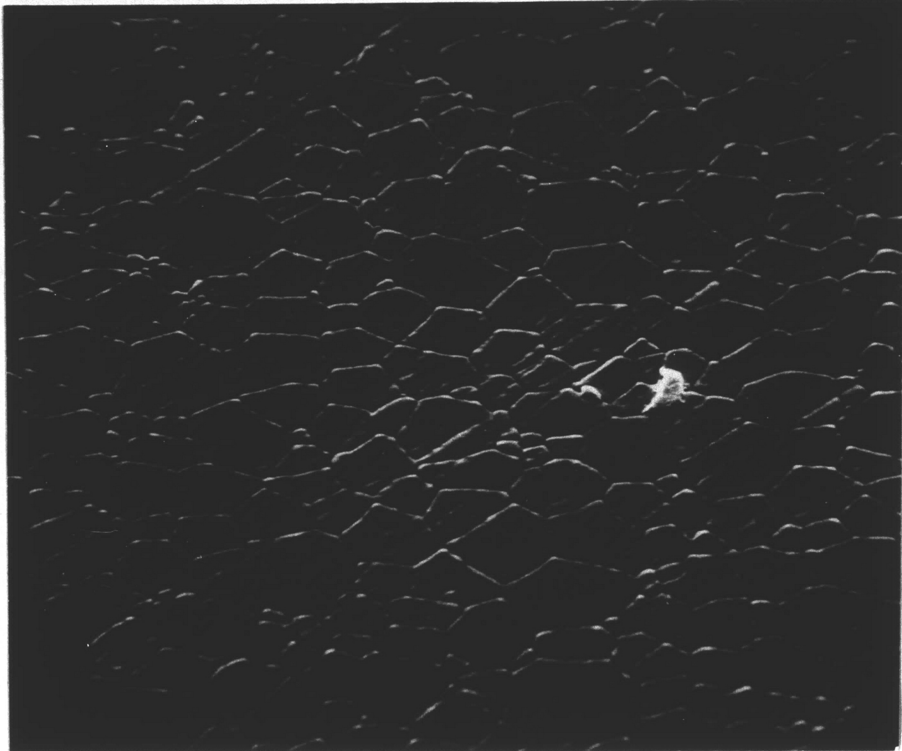
FIGURE 17 SCANNING ELECTRON MICROGRAPH SHOWING A TYPICAL HEAT TREATED SPECIMEN (1250°C-1,920 MINUTES) WHICH HAS BEEN THERMALLY ETCHED (2,100X)
