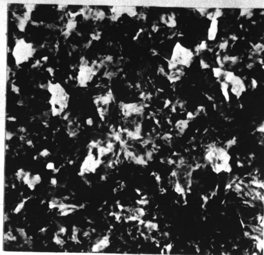
FIGURE 7 Etch: 1% Nital Mag: 250X Proof Stressed to 87% UTS, Stress Relieved 700°F, 8 hrs., A.C.
