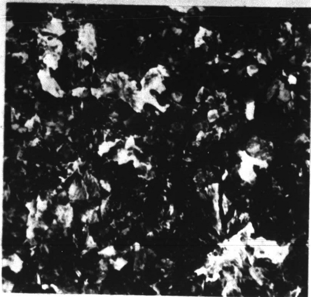
FIGURE 6 Etch: 1% Nital Mag: 250X Stress Relieved 700°F, 4 hrs., A. C., Proof Stressed to 87% UTS
