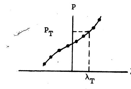
Now a different  $\lambda$  is selected, and the whole process repeated again to get another point on the graph. When enough points have been obtained, the multiplier  $\lambda_{T}^{}$ , which gives the desired total production  $P_{T}$  may be read off. This value of  $\lambda_{T}^{}$  is then used in each pair or equations (1) to solve for  $R_{i}$  and  $Q_{i}$ .
