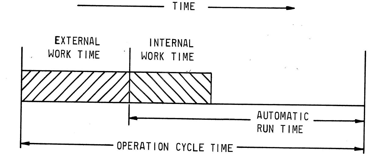
machine was non-productive. This type of work, conventionally called "external work", consisted of the unloading, loading and machine starting elements. The operator then immediately performed some "internal work" after the beginning of the machine's automatic production time.
