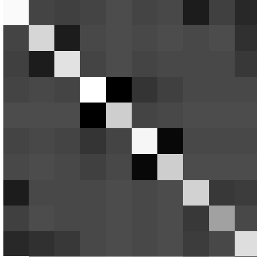
Figure 4.3: Gray scale pattern of susceptance of all links of power network, i.e., L .
