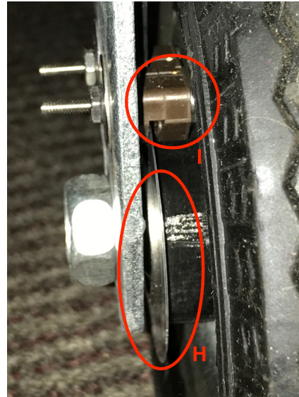
(b) Front fixed wheels with H) encoder disk, and I) encoder module
