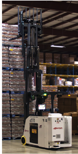
(a) AGV Forklift picking and dropping items
