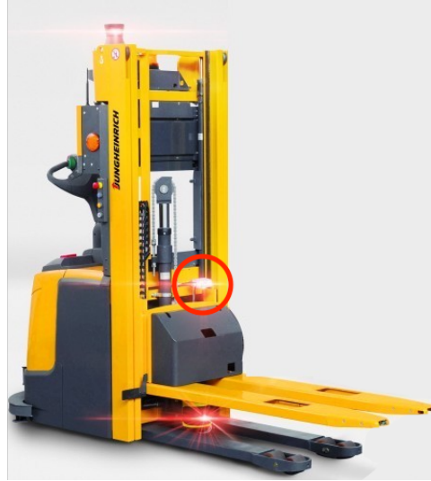
(b) AGV Forklift with LiDAR being used for pallet detection (encircled)
