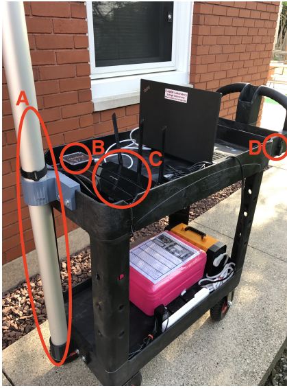
(a) 3D-DAC with all the components: A) telescopic mast, B) Puck Interface box, C) Wi-Fi router, D) Microstrain IMU
