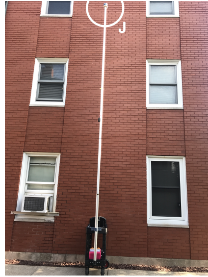
(b) 3D-DAC with fully extended, 6 m high telescopic mast
