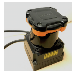
(c) Hokuyo UTM-30LX 2D LiDAR
