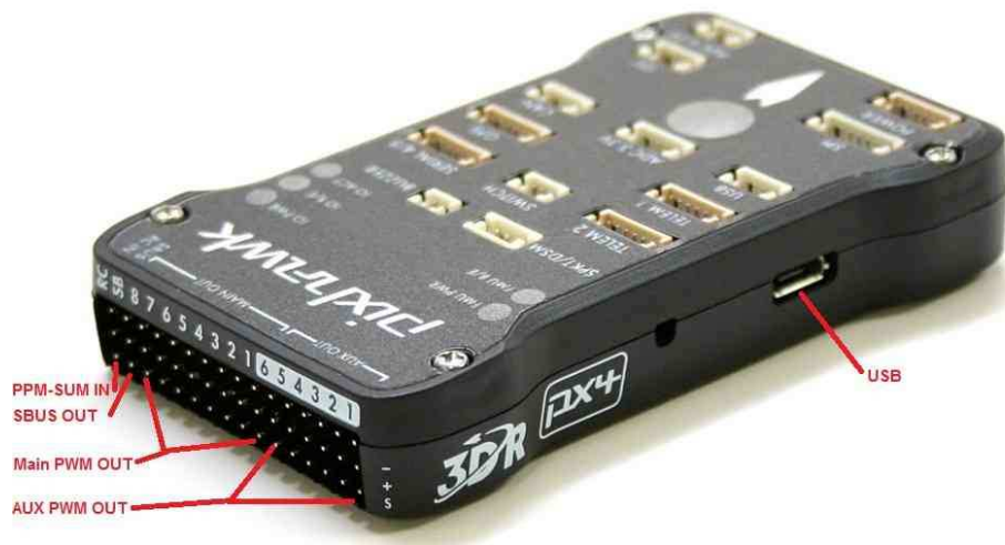
Figure 2.2: The Pixhawk connector pins.
