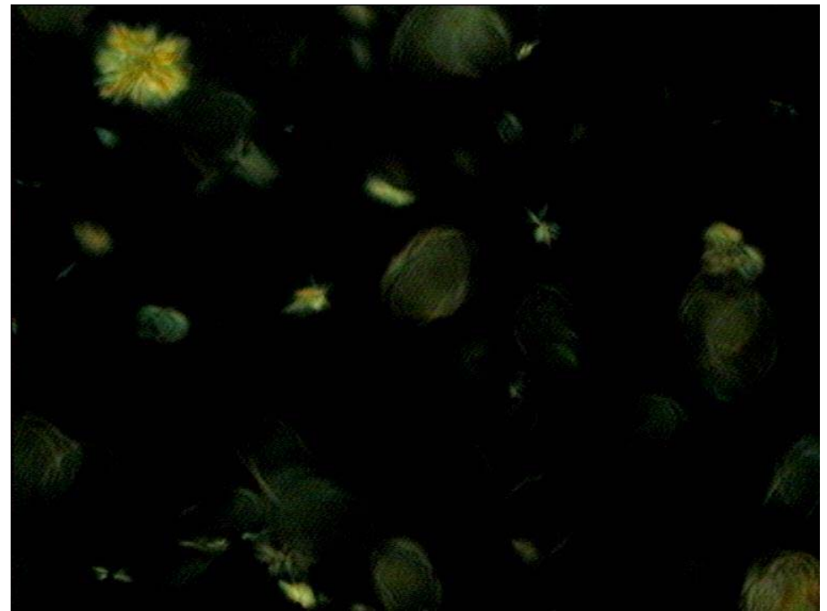
63°C, \Delta T=4\text{min} . Internal nucleation
