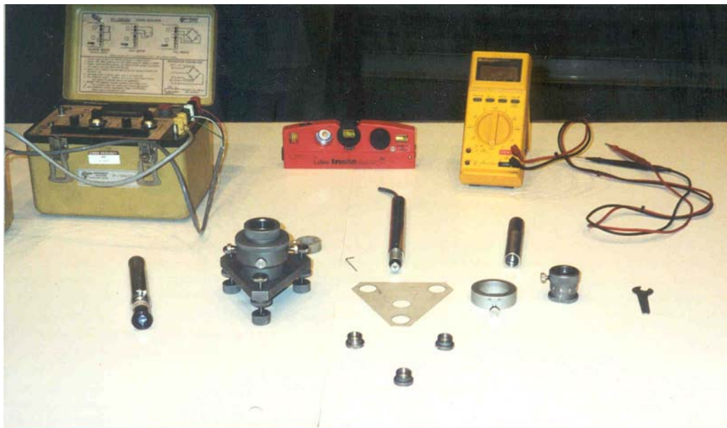
(b) Strain indicator and RS-200 Milling Guide Figure 4.40 Residual stress measurements
