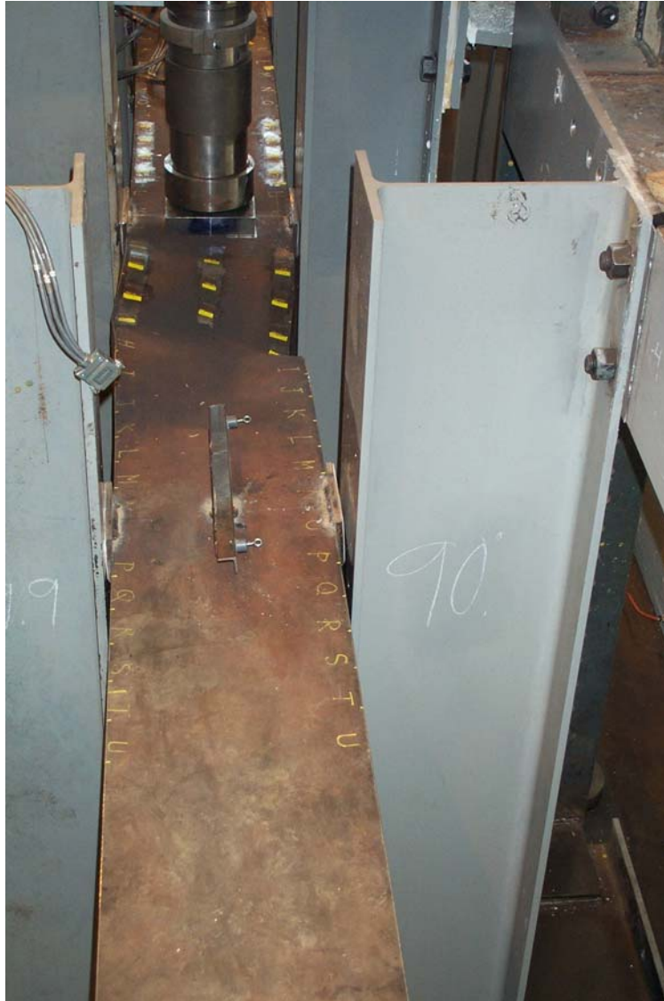
Figure 5.111 Lateral distortion of compression flange (Specimen 6)
