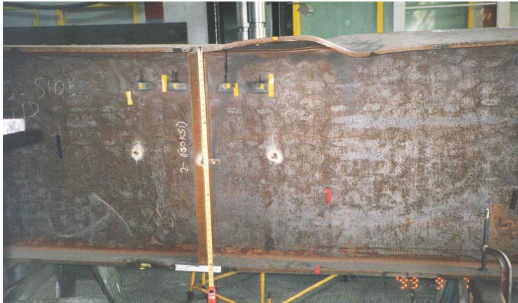
(b) Deflected shape after experiment
