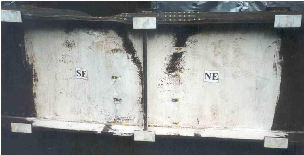
(b) Deflected shape from experiment
