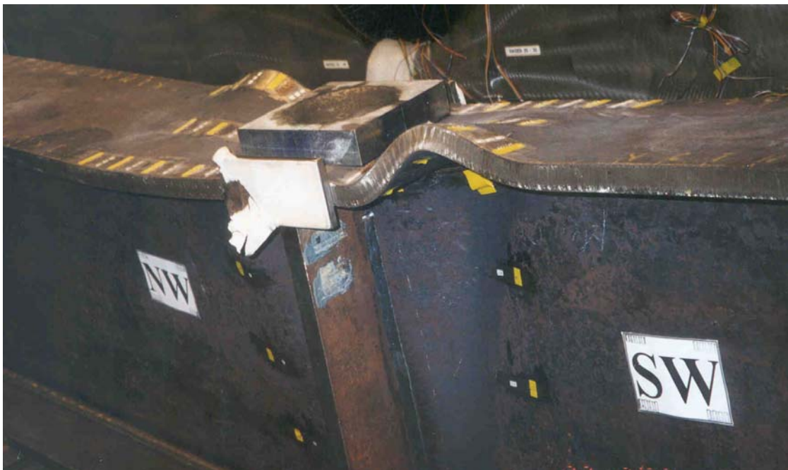
(b) Deflected shape from experiment
