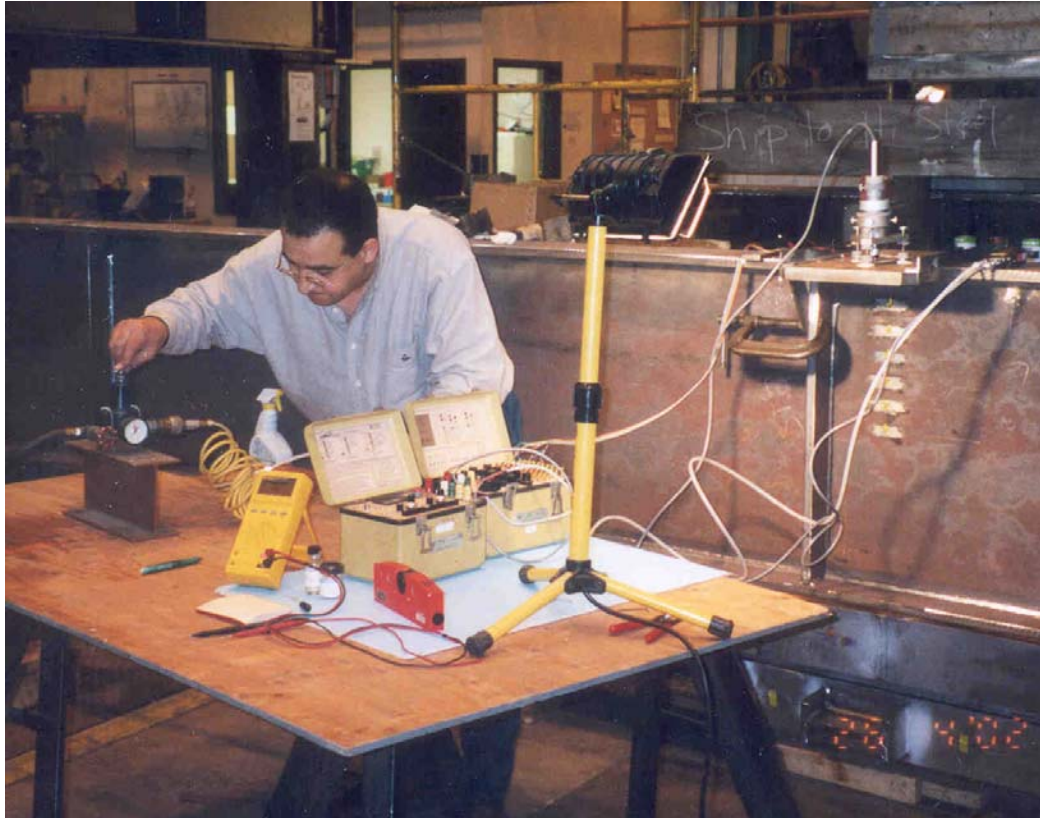
(a) Residual stress measurements using hole-drilling method
