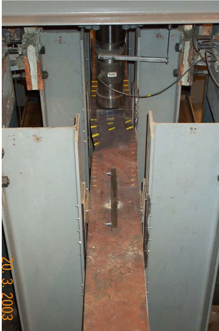
Figure 5.12 Lateral distortion of compression flange (Specimen 3)
