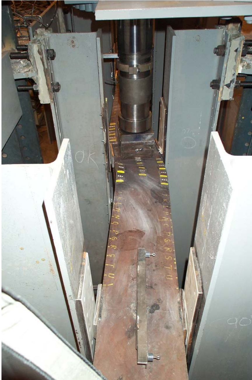
Figure 5.86 Lateral distortion of compression flange (Specimen 5)
