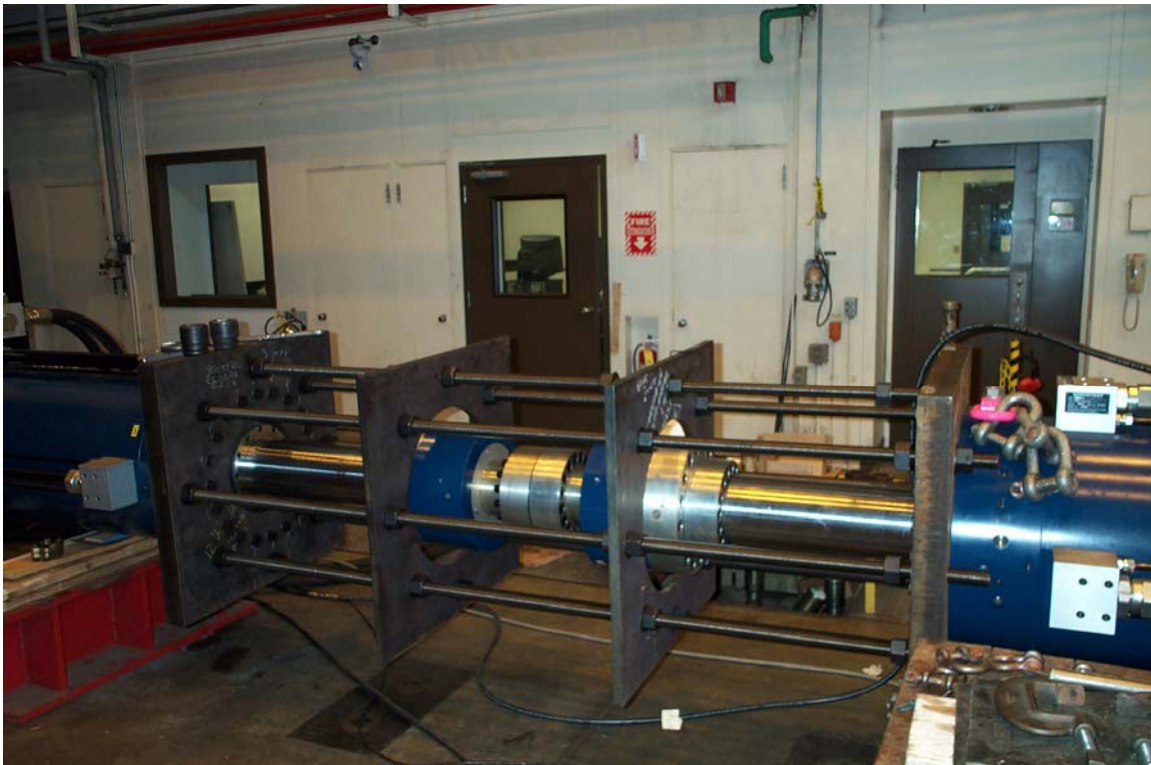
Figure 5. Test power with displacement actuator and load actuator
