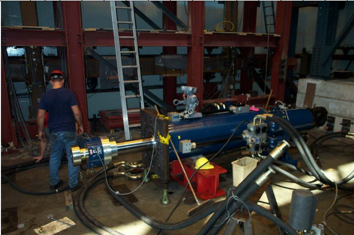
Figure 4. Free-standing servo actuator for Test 1, 2, and 3
