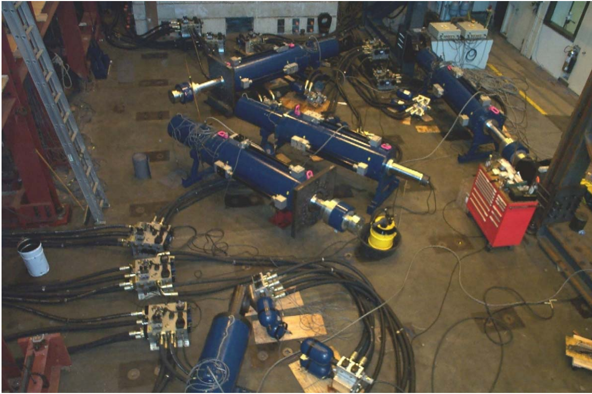
Figure 2.3.2 Deployment of the accumulator system test
