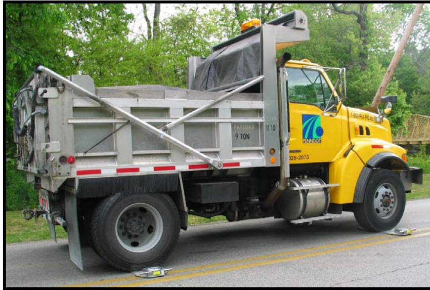
Figure 3.1 – The single axle truck (lighter truck) used in the controlled load testing
