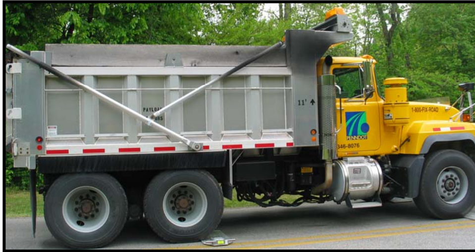
Figure 3-2 – The tandem axle truck (heavier truck) used in the controlled load testing
