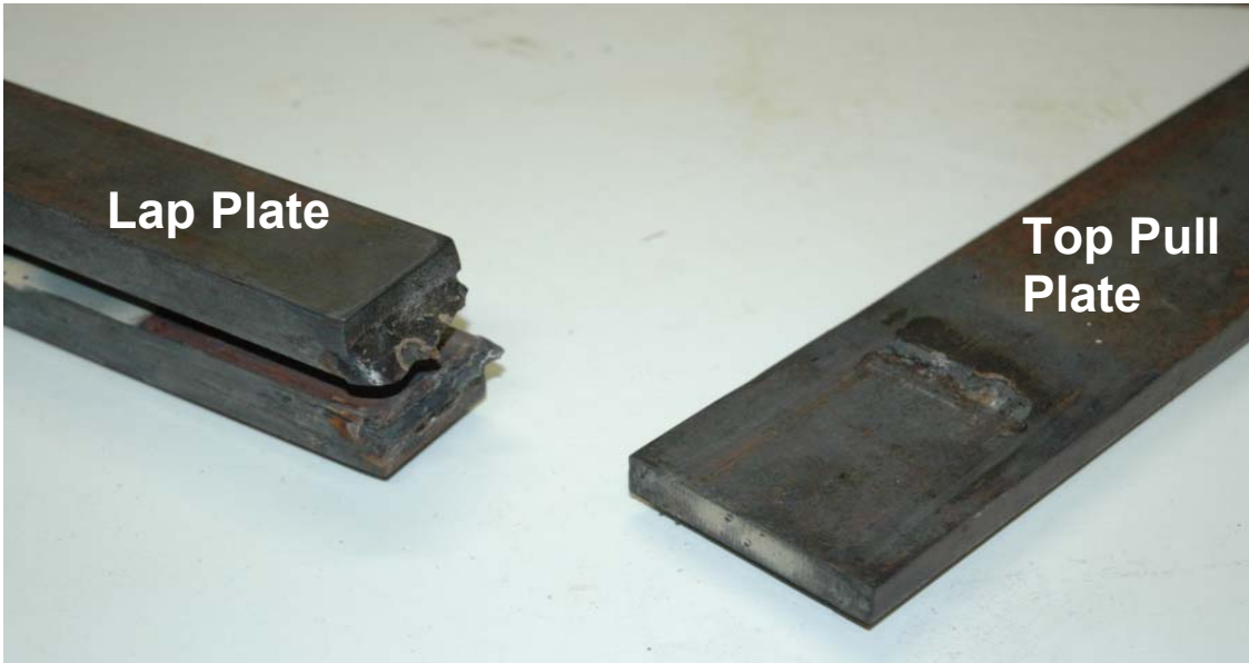
Figure 4.26 Photograph of Specimen 7 after fracture, where the weld on the lap plate and top base plate is visible
