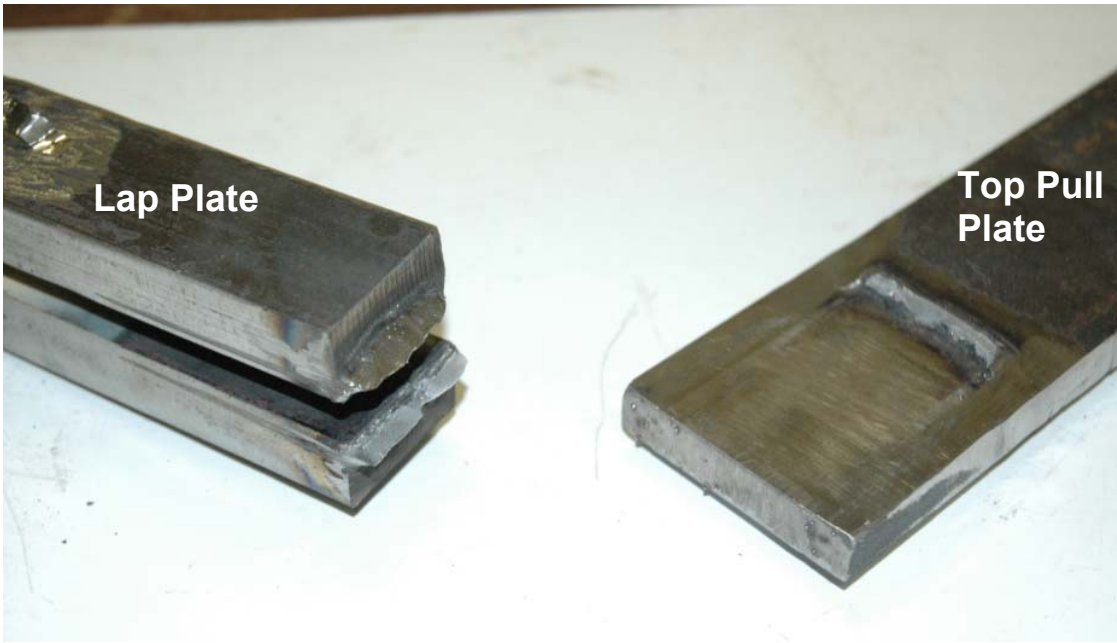
Figure 4.2 Photograph of Specimen 1 after fracture, where the weld on the lap plate and top base plate is visible
