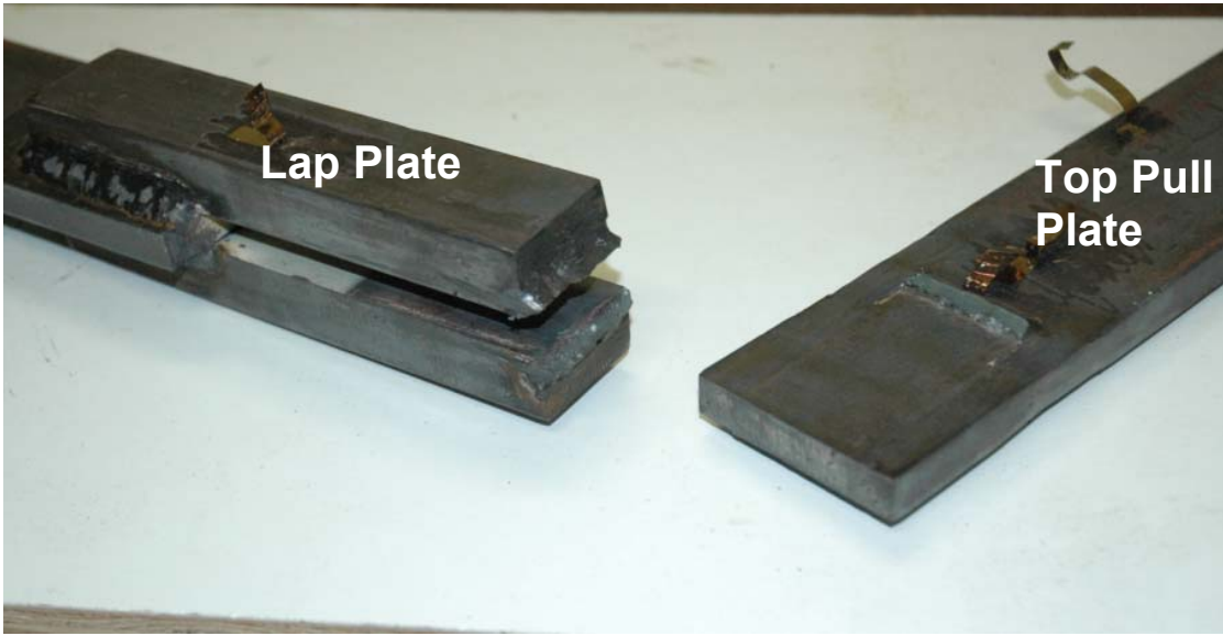
Figure 4.18 Photograph of Specimen 5 after fracture, where the weld on the lap plate and top base plate is visible
