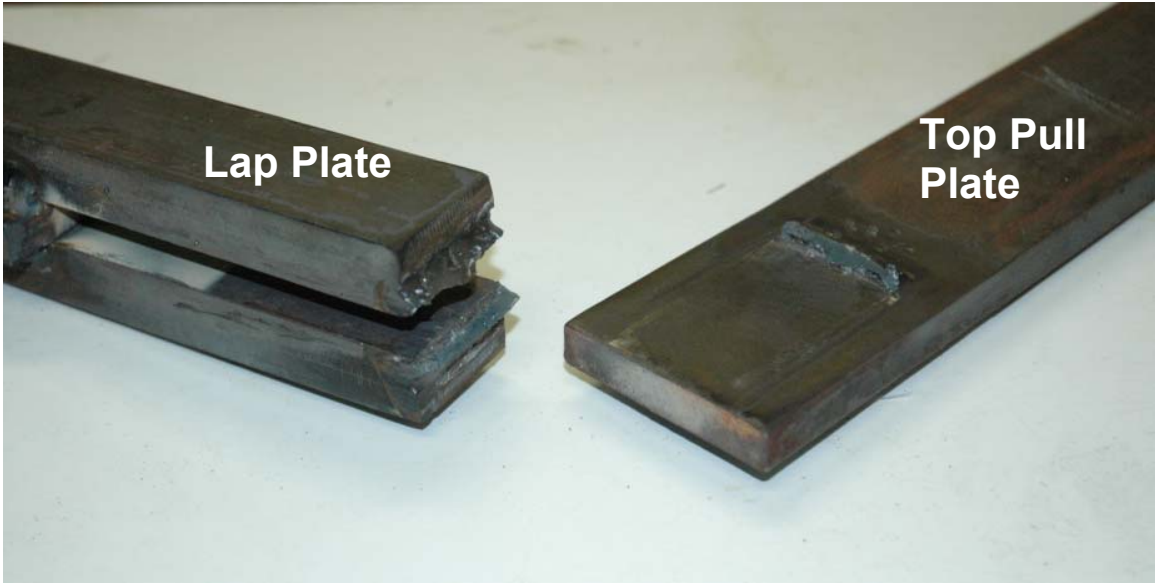
Figure 4.14 Photograph of Specimen 4 after fracture, where the weld on the lap plate and top base plate is visible
