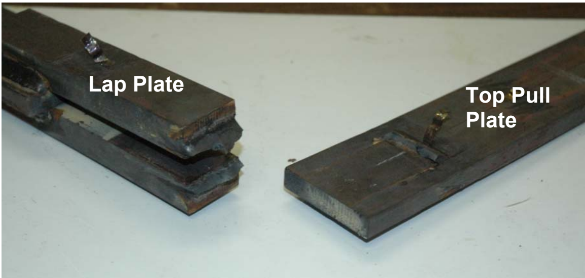
Figure 4.22 Photograph of Specimen 6 after fracture, where the weld on the lap plate and top base plate is visible
