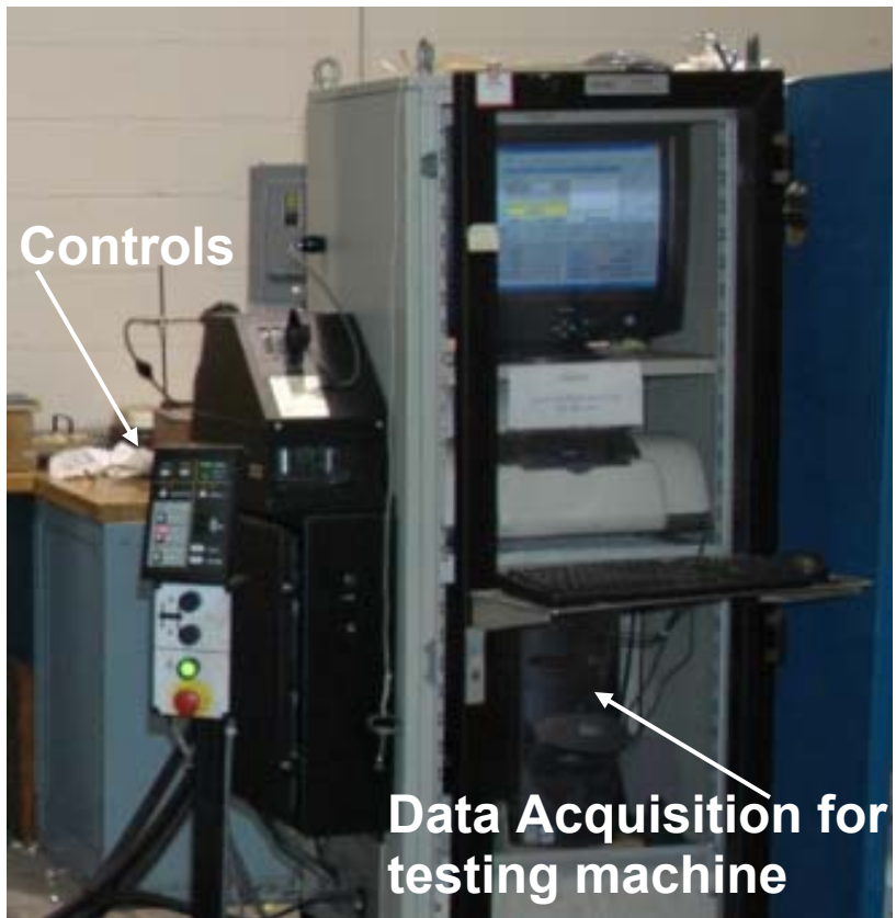
Figure 3.12 Photograph of the controls and data acquisition for the SATEC testing machine
