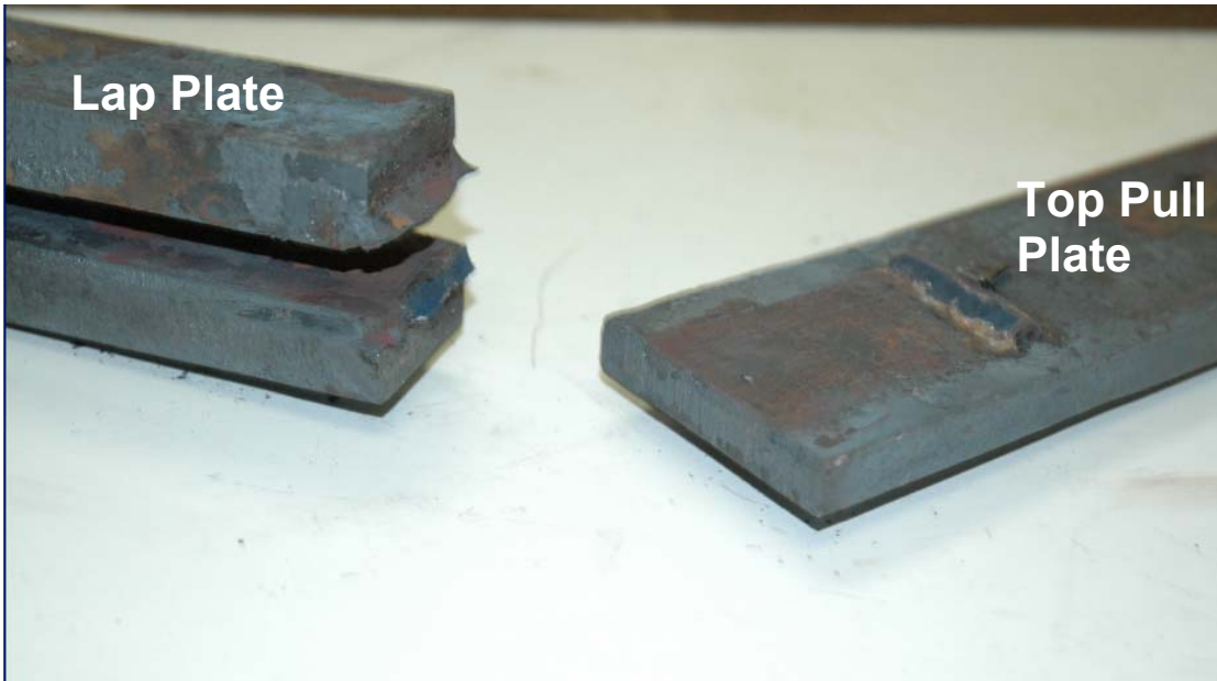
Figure 4.44 Photograph of Specimen P2 after fracture, where the weld on the lap plate and top base plate is visible
