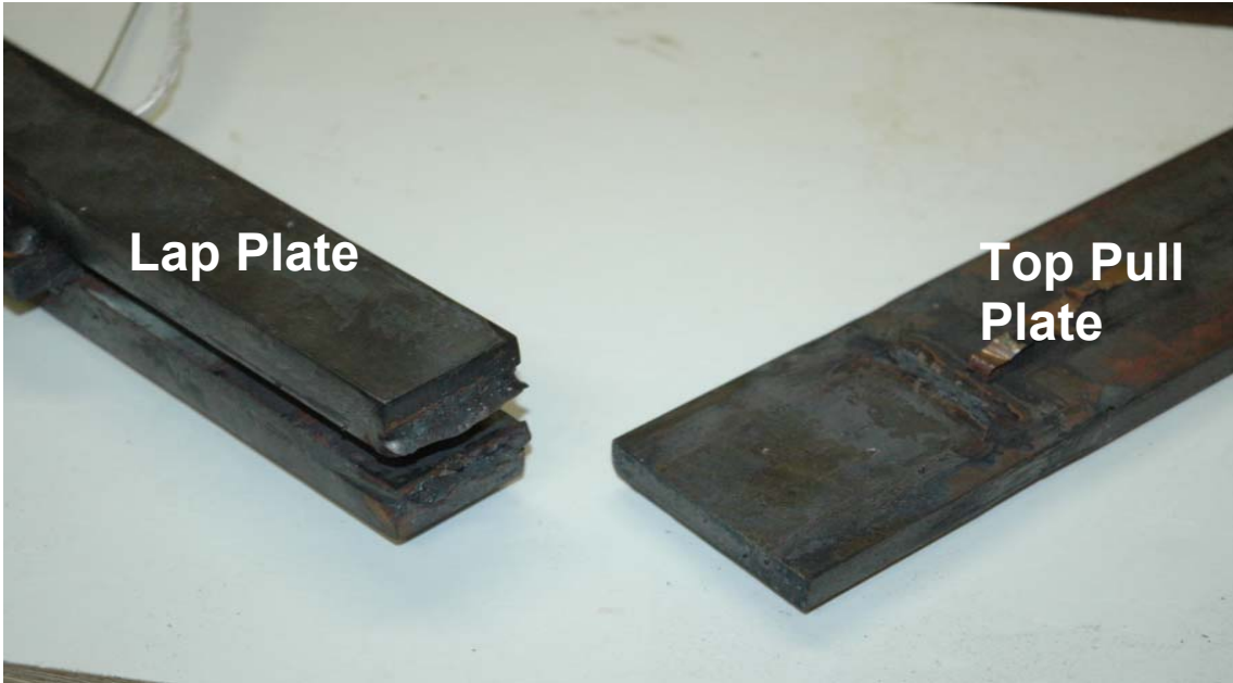
Figure 4.30 Photograph of Specimen 8 after fracture, where the weld on the lap plate and top base plate is visible
