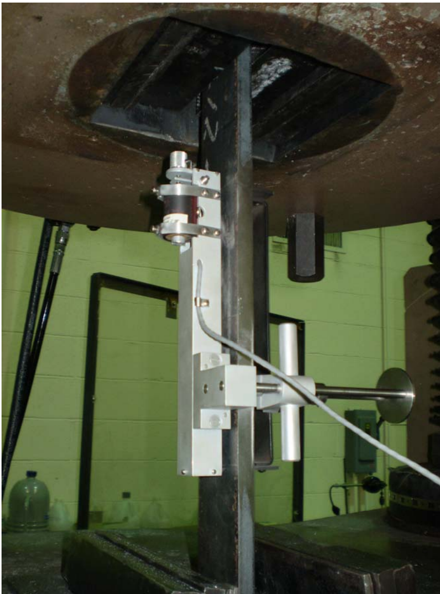
Figure 3.15 Photograph of bar and extensometer in testing machine
