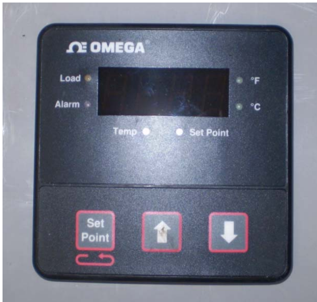
Figure 3.11 Photograph of digital temperature controller
