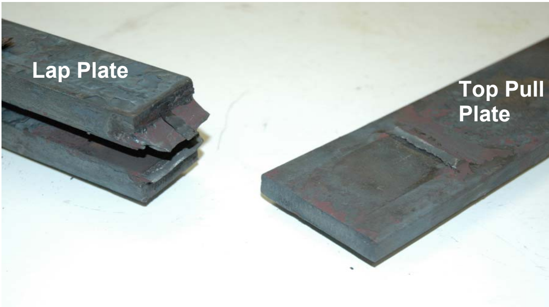
Figure 4.48 Photograph of Specimen P3 after fracture, where the weld on the lap plate and top base plate is visible
