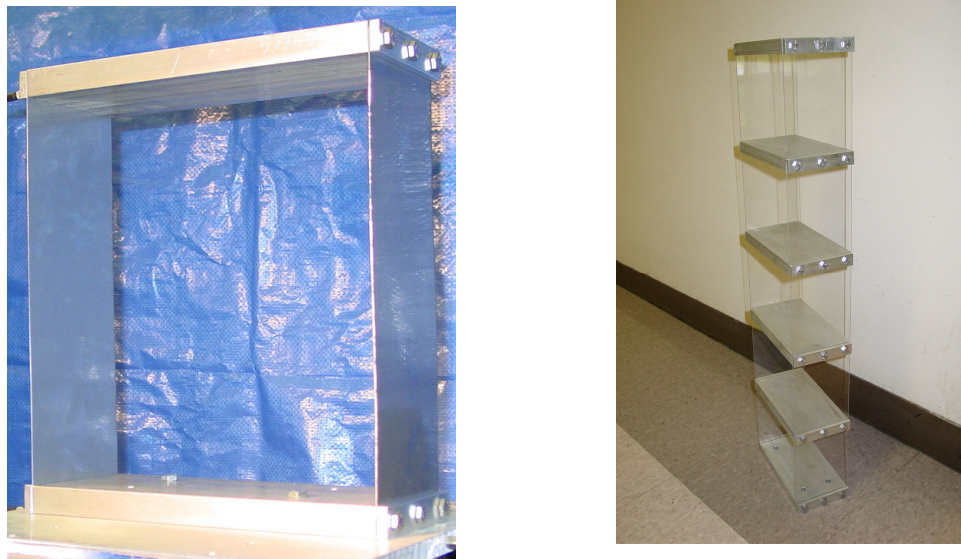
Figure 2: 1-Story and 5-Story Model Structures
