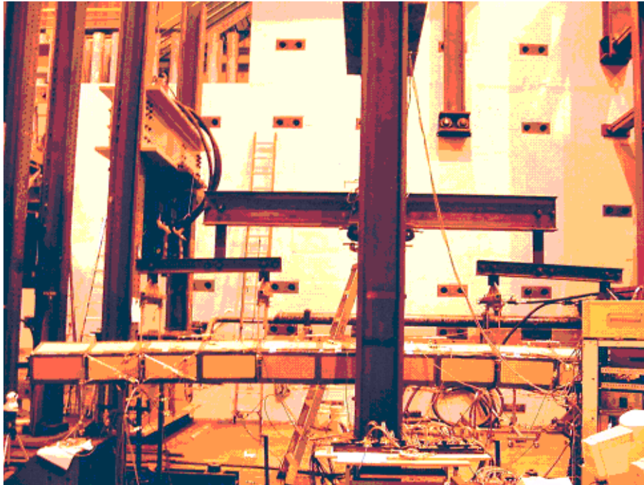
Fig. 13. Sagging test with load at 40% above the design load. There is substantial deflection, containing both elastic and plastic parts.
