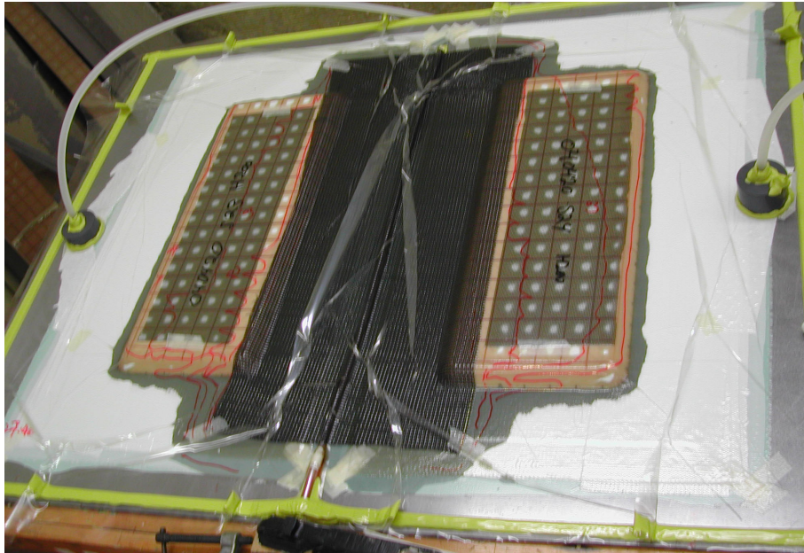
Fig. 4. Vacuum infusion process for a composite sandwich panel.
