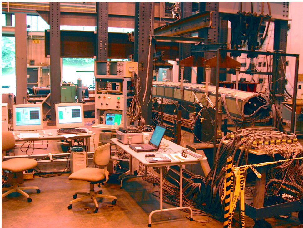
Fig. 12. Data acquisition system.
