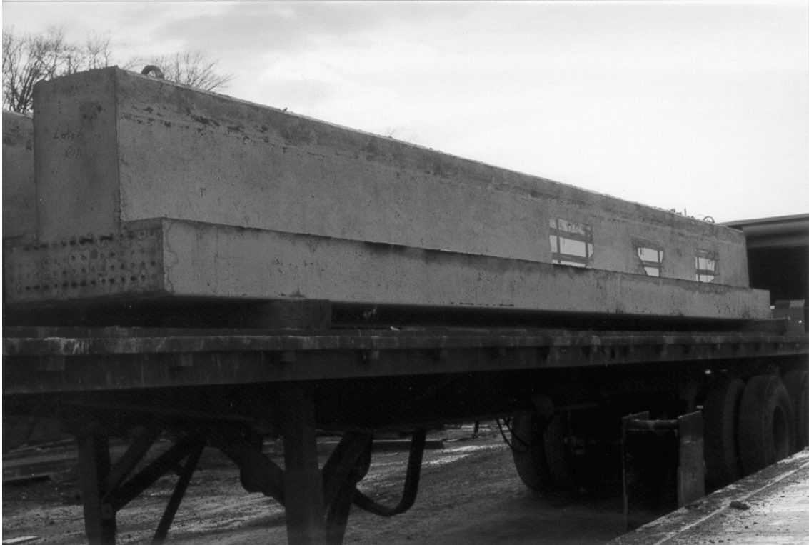
Figure 2.10 Specimen after initial curing and transfer of prestress
