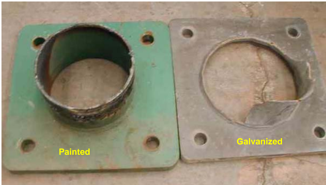
Figure 2.2 – Baseplates of sign poles
