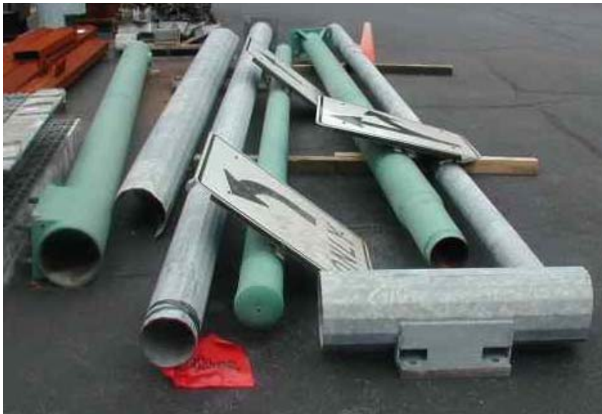
Figure 2.1 – Components of sign structures delivered to the ATLSS Center (Poles referred to as “painted” are the green components)
