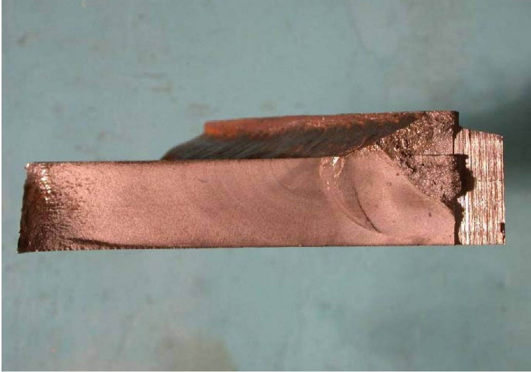
Figure 27. Fracture surface from Girder G4A.
