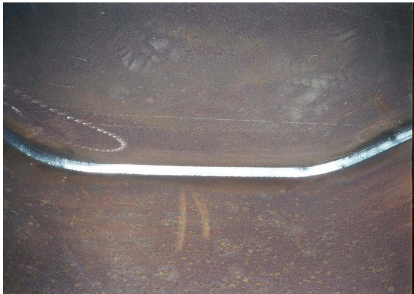
Figure 9. Robotically made fillet weld.
