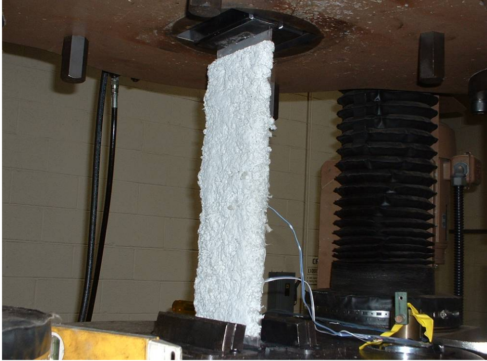
Figure 3.7 – Plate specimen installed in universal testing machine
