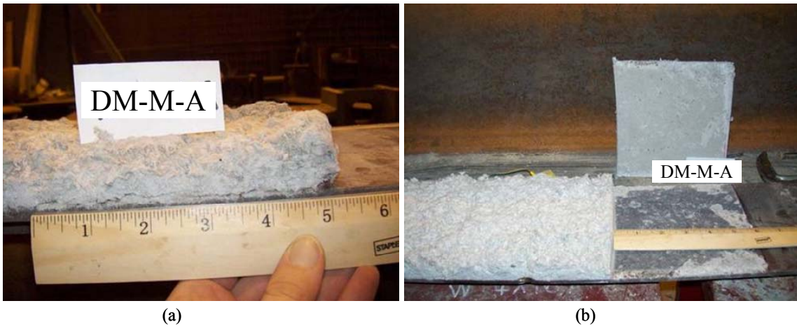
Figure 4.8 – DM behavior due to post-yield strain loading: (a) detachment of DM at one end; and (b) lack of adhesive strength after first cut is made into the DM
