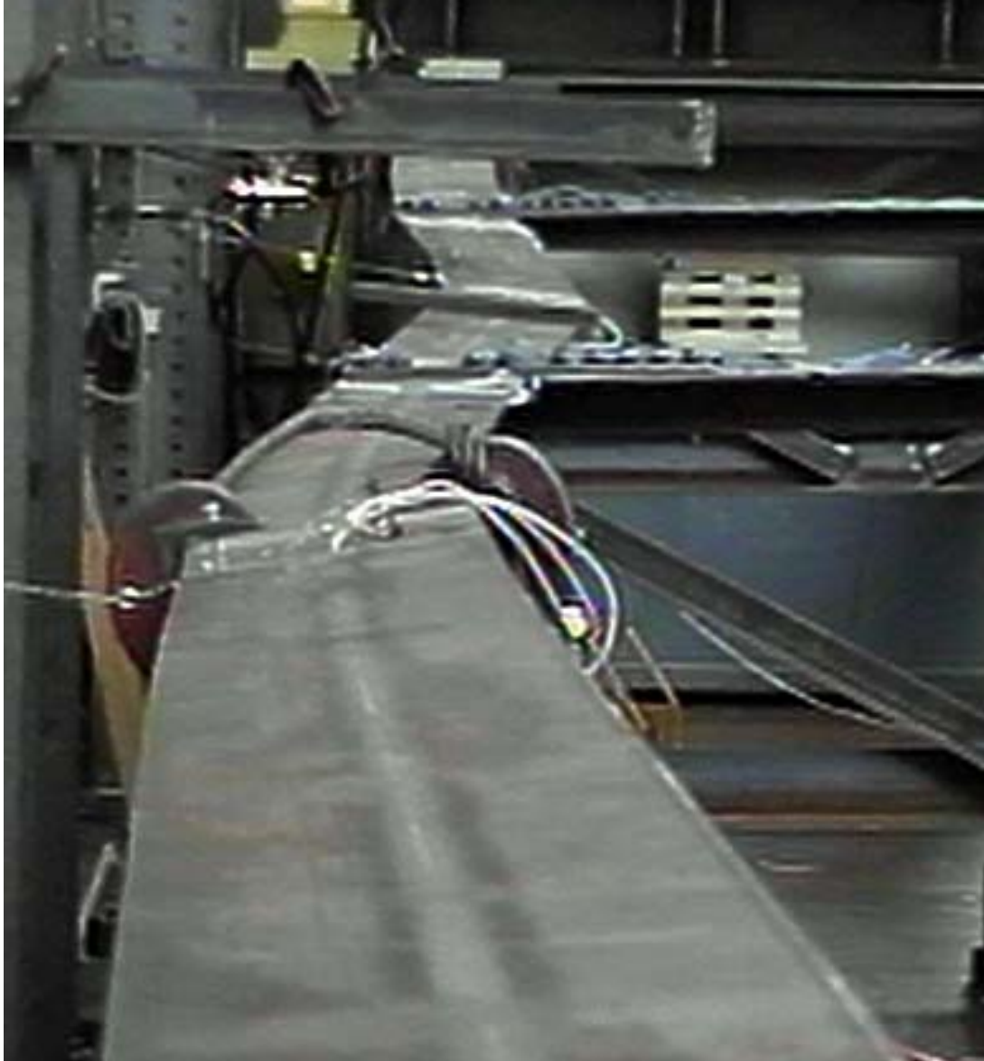
Figure 22. Photograph of north girder after peak load.
