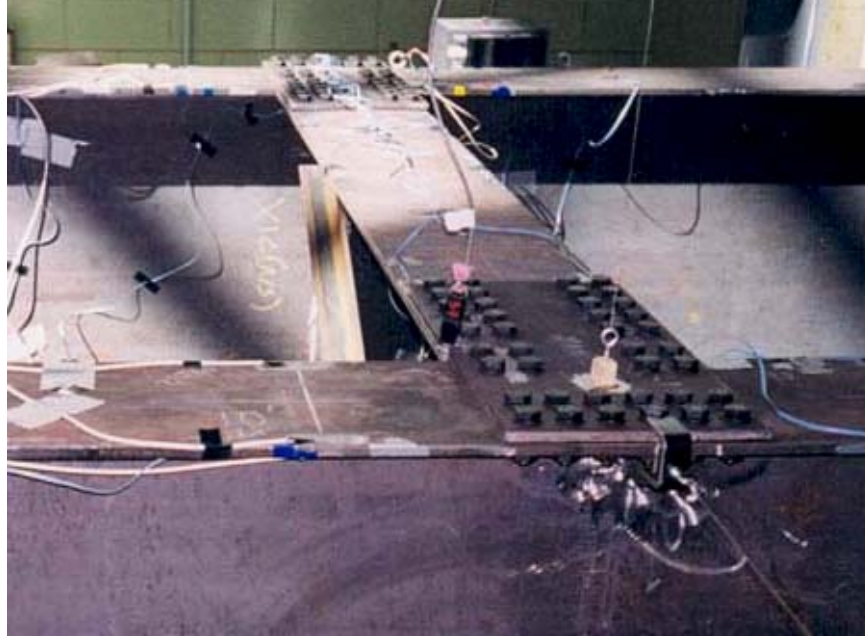
Figure 1. FRRB used in test specimen.
