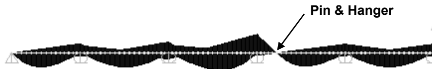
Figure 5 – Moment envelope for pin and hanger model (half length)
