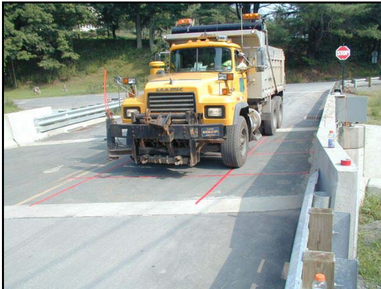
Figure 11.1 – Photograph of test truck #2 (107-8076) utilized during controlled load testing
