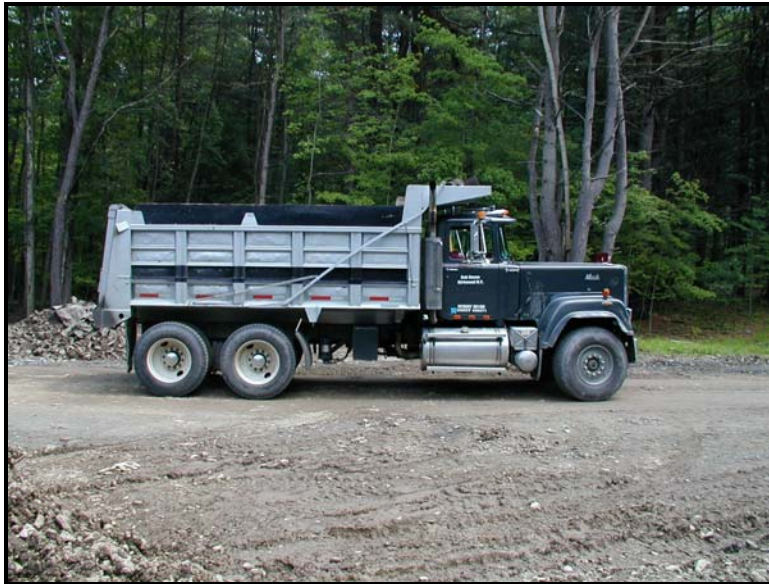
Figure 3.1 – Photograph of test truck utilized during the controlled load tests
