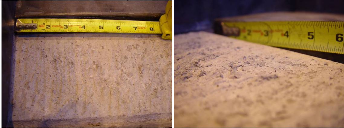
Figure 9-14: Rake Surface Finish – “Intermediate” [Specimen 6R6]
