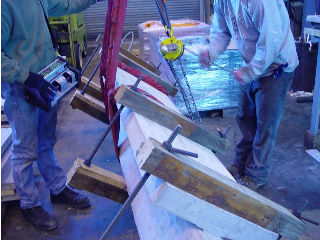
Figure 8-10: Flipping the Test Specimen
