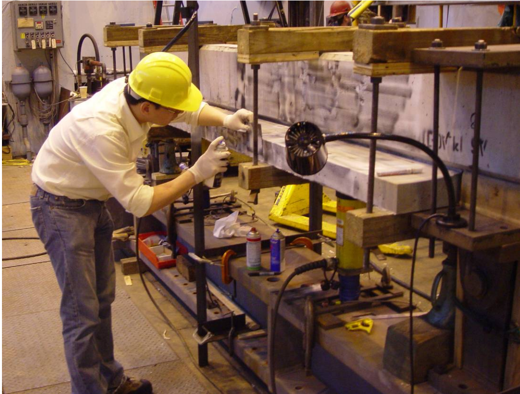
Figure 8-28: Applying Pattern to the Slab Concrete with Spray Paint [Specimen 6A8]
