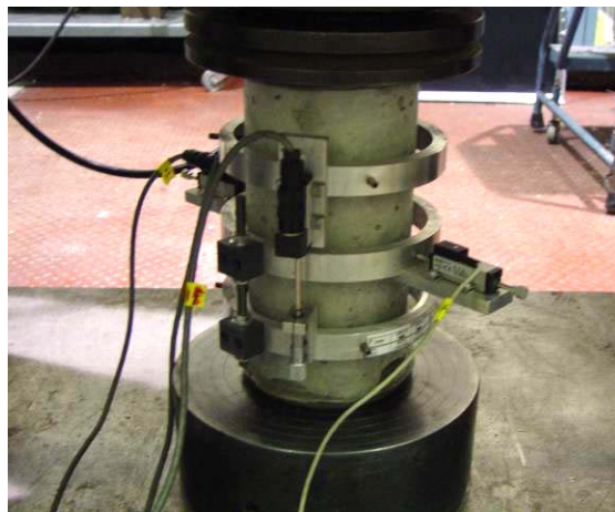
Figure 8-33: Test Frame and Test Setup for a 6x12 Cylinder
