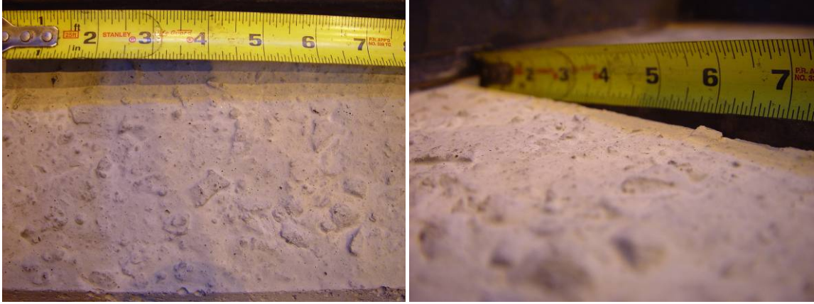
Figure 9-11: As-Placed Surface Finish – “Intermediate” [Specimen 6A5]
