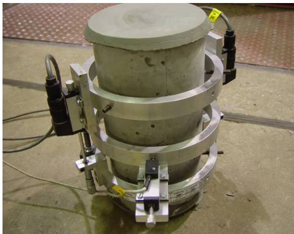
Figure 8-33: Test Frame and Test Setup for a 6x12 Cylinder
