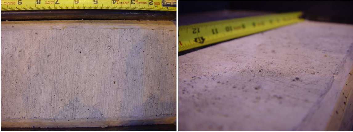
Figure 9-9: Broom Surface Finish [Specimen 6B6]
