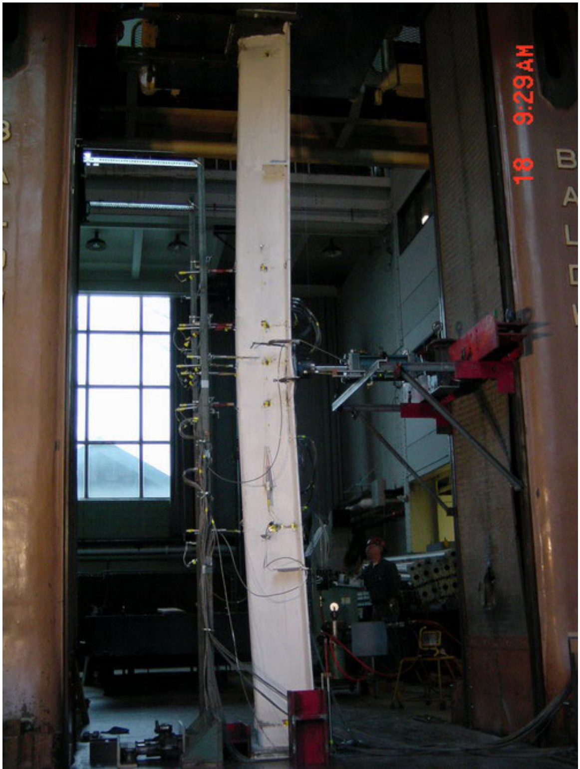
Figure 4-15 Final Appearance of Single Rib Beam-column Specimen SBC1
