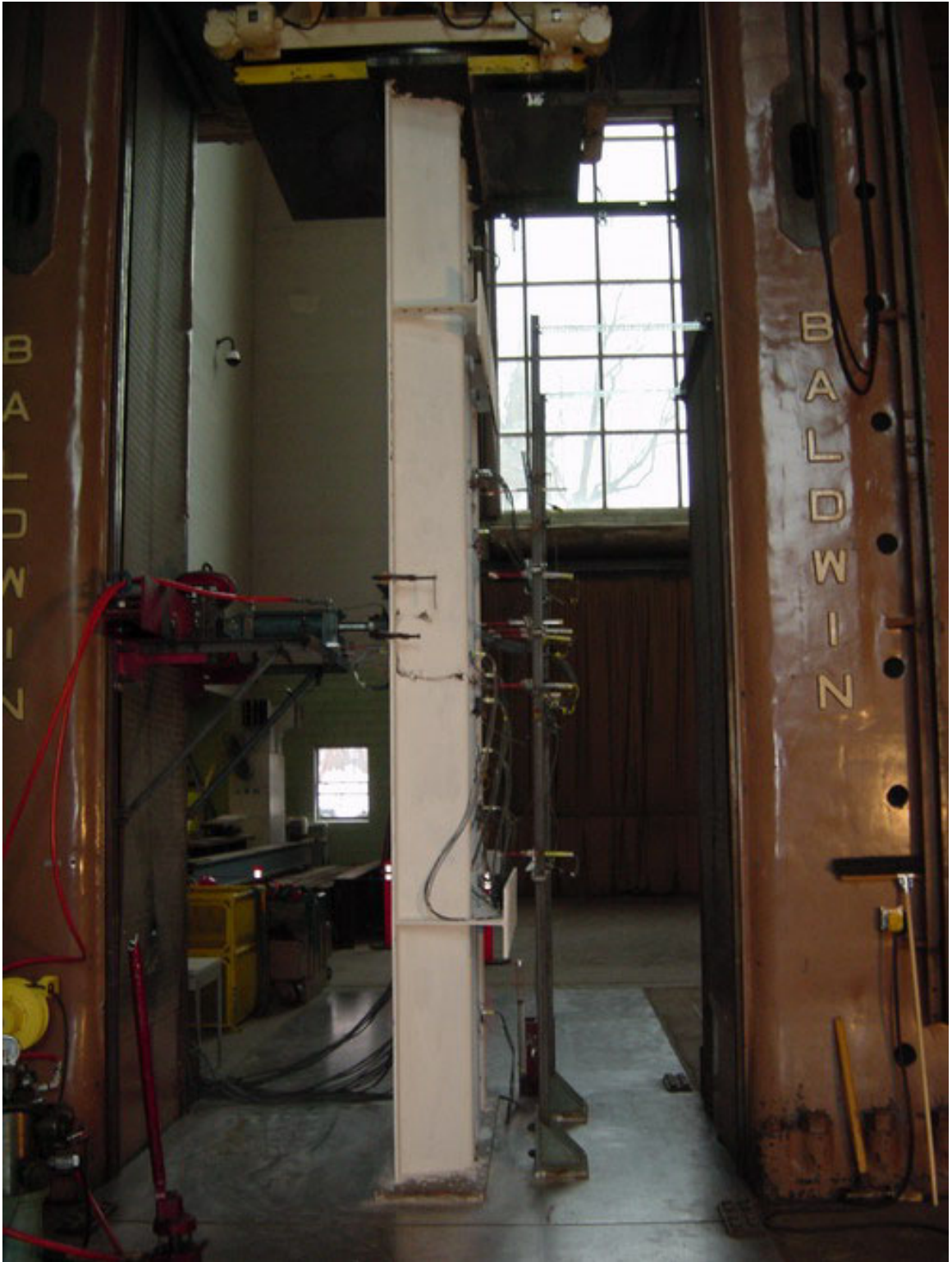
Figure 4-21 Final Appearance of Triple-rib Beam-column, TBC
