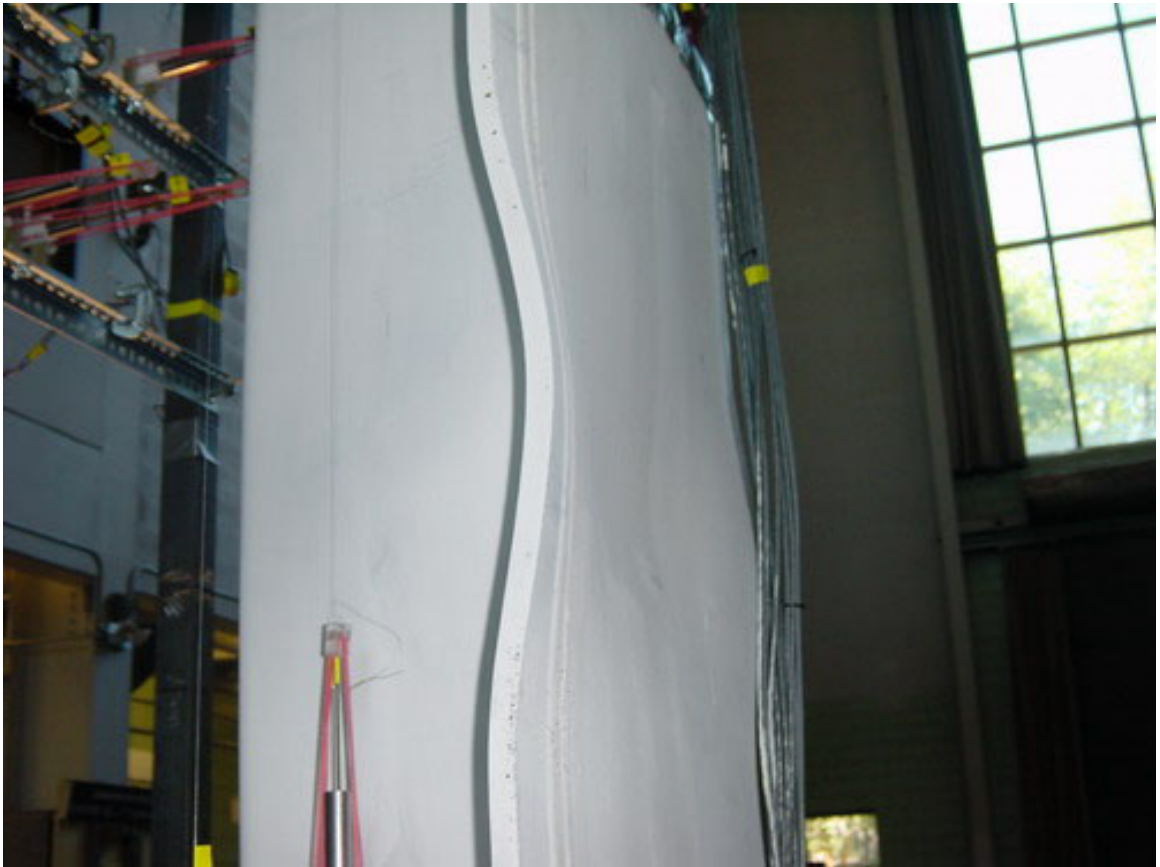
Figure 4-14 Local Buckling of Deck Plate near Mid-height of Single-rib Column, SC
