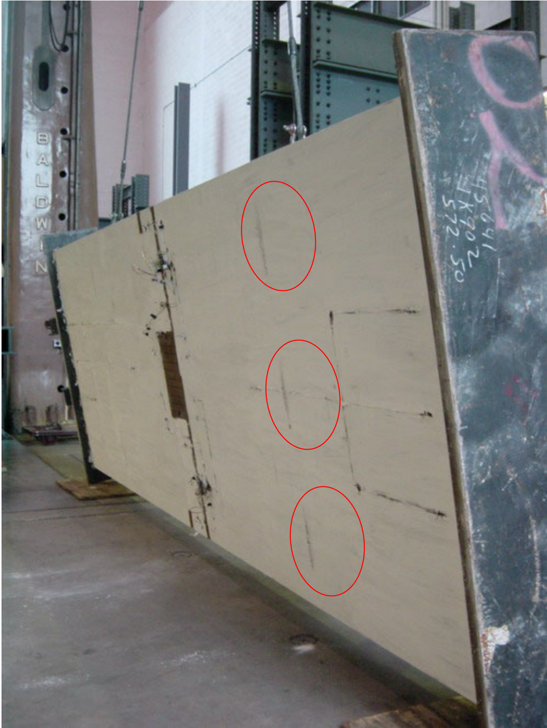
Figure 4-22 Yielding Lines on Deck Plate of Triple-rib Beam-column, TBC
