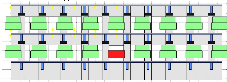
Figure 4-20: View of the center wall of Analysis 2 showing the bottom opening position and the burning vehicle centered in between the double-tee stems.
