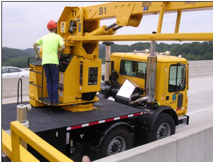
Figure 3.15: Aspen Aerial UB50 snooper used for instrumentation of bridge
