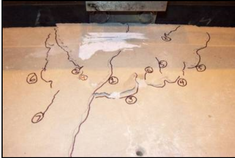
Figure 83: Altus slab top surface crack patterns (near end of test)
