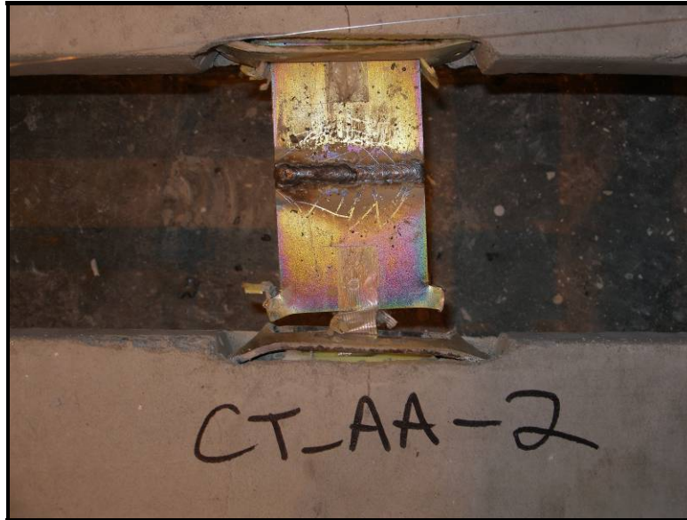
Figure 56: Specimen CT_AA-2 – after fracture of connector at a displacement of 3.6 inches
