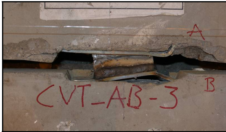
Figure 70: Specimen CVT_AB-3 – deformation of the “B” connector face plate at a shear load of 4.1 kips and a tension load of 1.1 kips (shear displacement of 0.3 inches)
