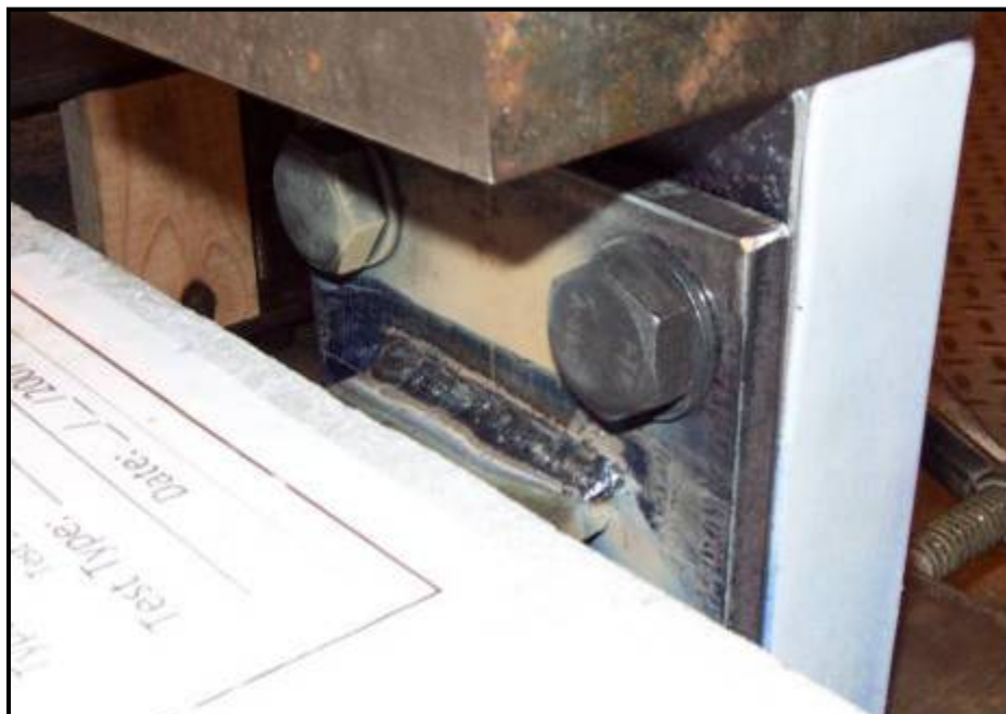
Figure 14: Out-of-plane tests – detail showing a Type A tab welded to the loading block
