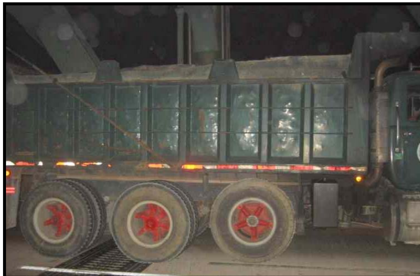
Figure 3.2 – Side view of the test truck showing the floating axle in the up position
